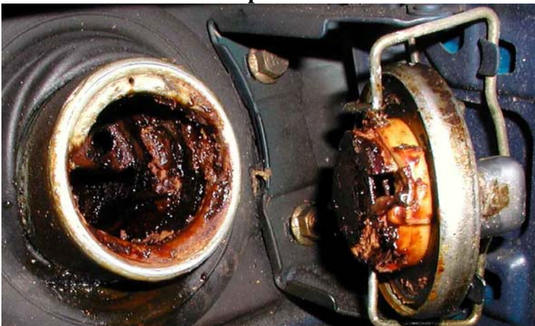
PHOTO 3. Fuel Tank Deposits
