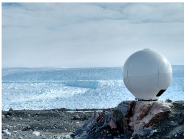
Fig. 1. TRI set-up at Jakobshavn Isbræ, Greenland. The instrument is inside the radome, the height of the radome is \sim 3 m. The calving front is \sim 3 km away.
