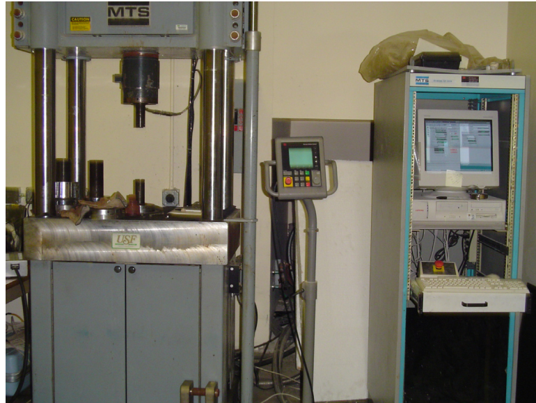
Fig 4.8 MTS Press Used for Preparing 2.0” Diameter Pellet
