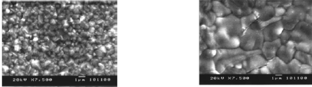
**Figure 12. SEM of As deposited (Left) and CdCl<sub>2</sub> Treated (Right) CdTe/CdS/O/Poly**
