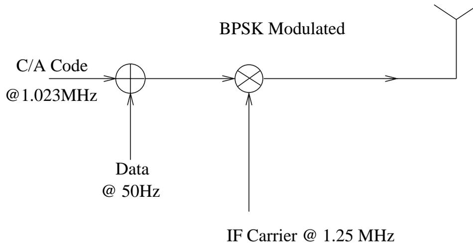
Figure 4.5. IF GPS Signal Generation
