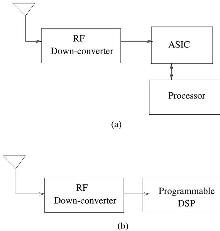
Figure 1.2. Receiver Block Diagrams: (a) Hardware (b) Software
