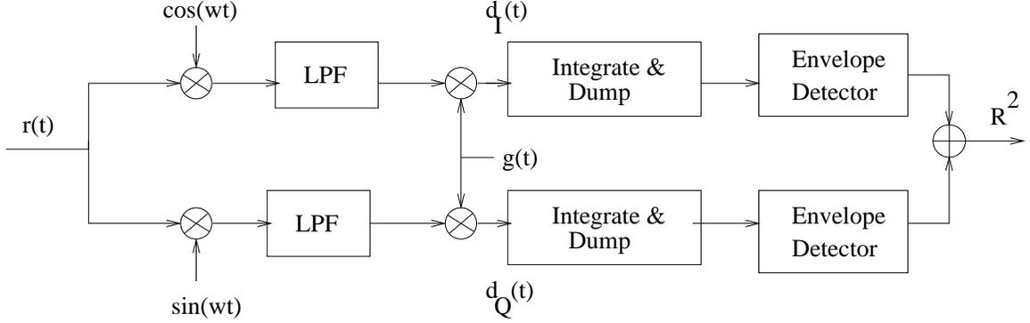
Figure 2.9. Non-coherent Demodulation
