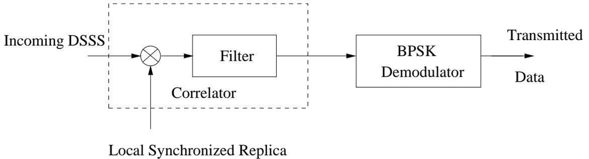
Figure 2.3. Direct Sequence Demodulator
