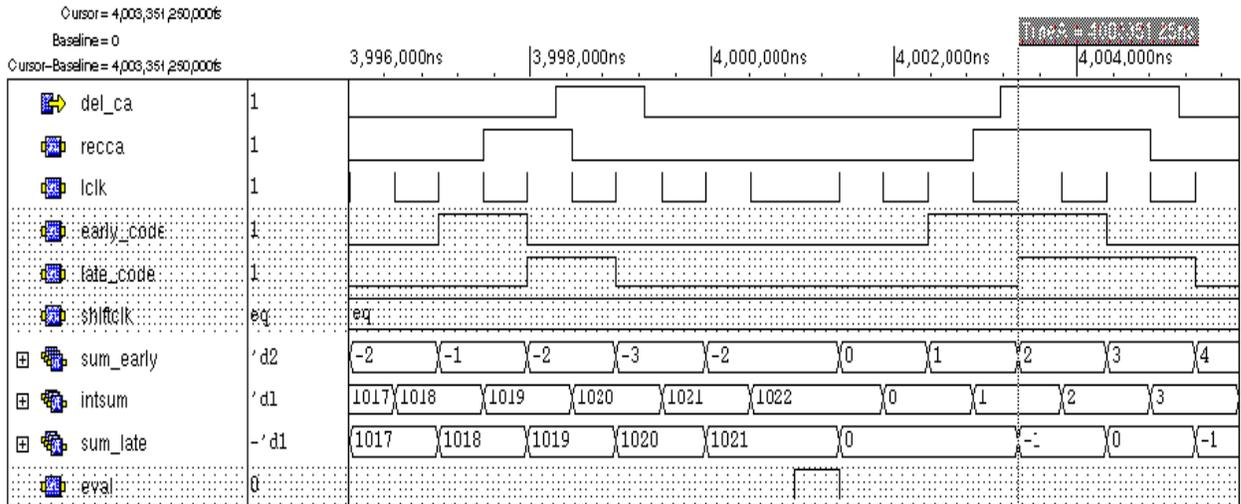
Figure 5.12. Tracking After Signal has been Acquired
