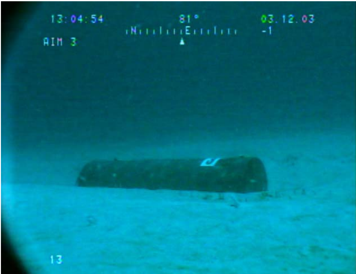
Figure 15. ROV video still image of the A3 mine on March 13, 2003. Camera is facing east-northeast showing a side view of the mine within the scour pit.
