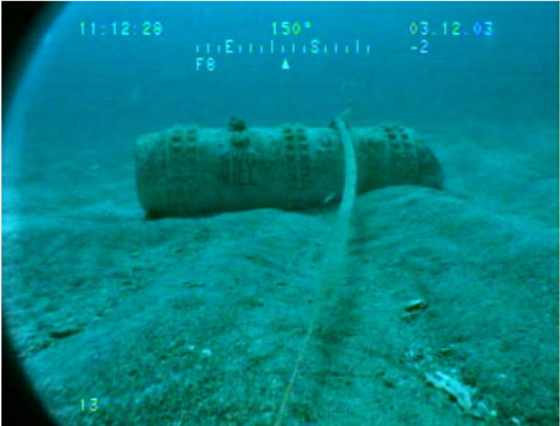
Figure 23. ROV video still image of the F8 mine on March 13, 2003. Camera is facing south-southeast showing a side view of the mine in the ripple field.
