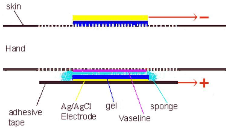
Figure 4. TransQ-1GS Ag/AgCl electrodes from Pro-Med.
