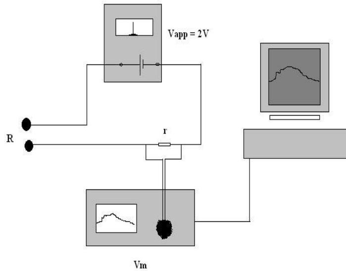
Figure 3. Schematic diagram of circuit and equipment used in the skin conductance study experiments.
