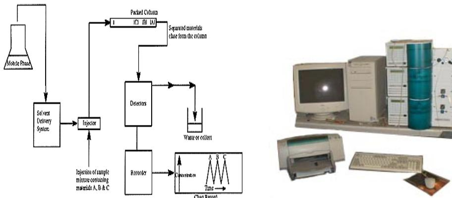
Figure 9. The components of HPLC instrument and the instrument itself.
