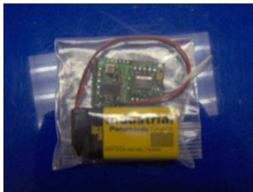
Figure 3.9 Accelerometer's y – axis Aligned with the Gravity Vector and Enclosed in a Plastic Bag.
