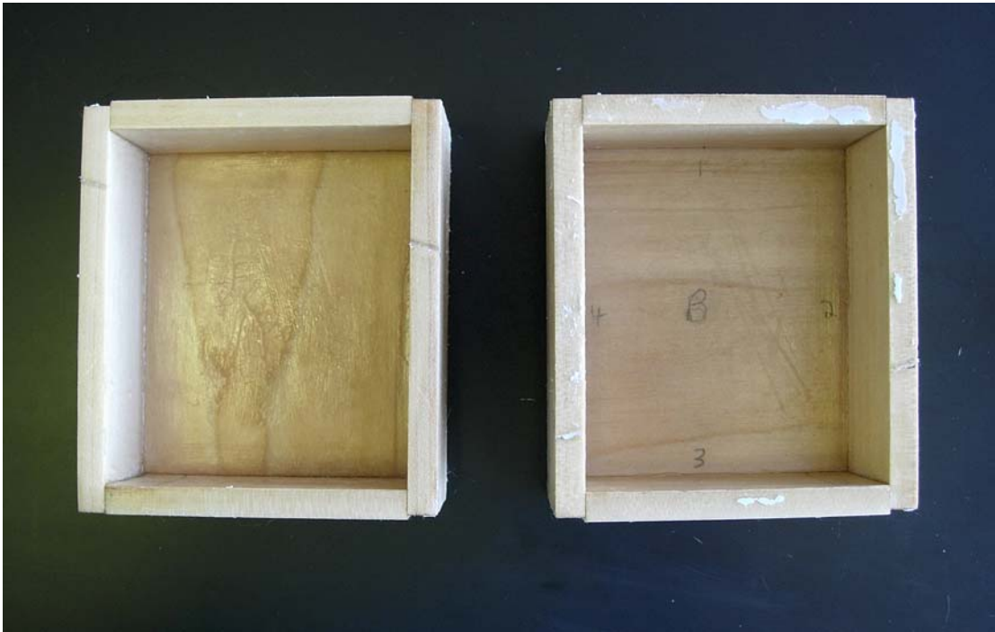
Figure A.4 – Box fabricated for pouring the silicone rubber molding. The box was held together by epoxy.
