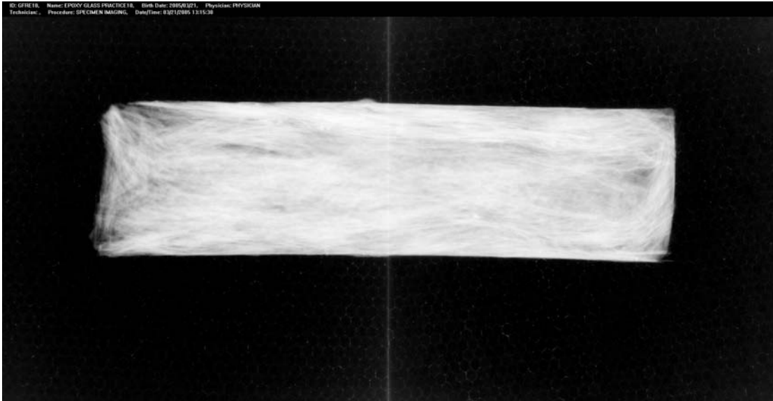
Figure A.9 - Ten vol% GFRE beam X-ray image used to estimate fiber orientation. Fiber orientation of the 10 vol% GFRE was largest in the length wise direction of the beams.
