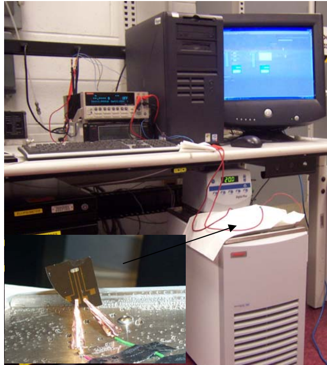
Figure 4.6 Measurement setup to measure temperature and resistance using labview
