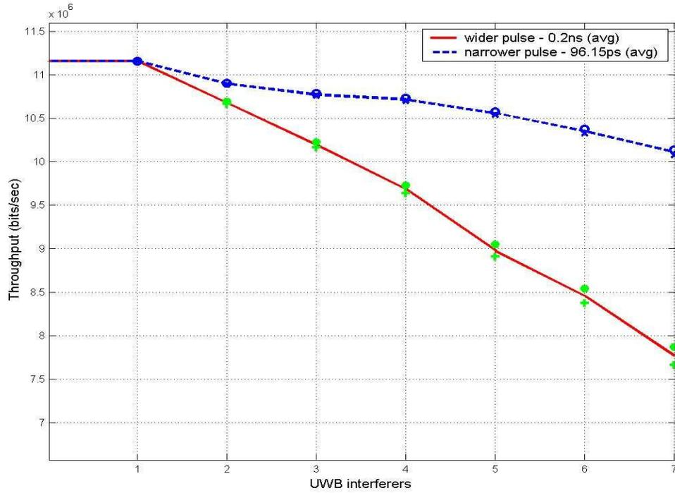
Figure 37. Throughput vs UWB Interferers (PW, STA to AP – 14 m, NM)
