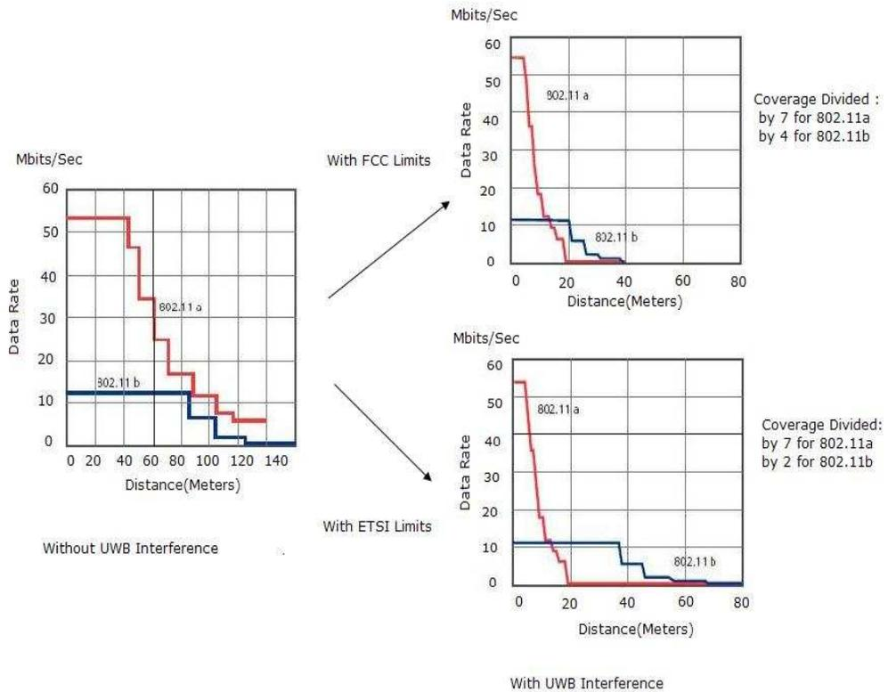
Figure 6. UWB Interference to IEEE 802.11a and IEEE 802.11b. Courtesy [17]
