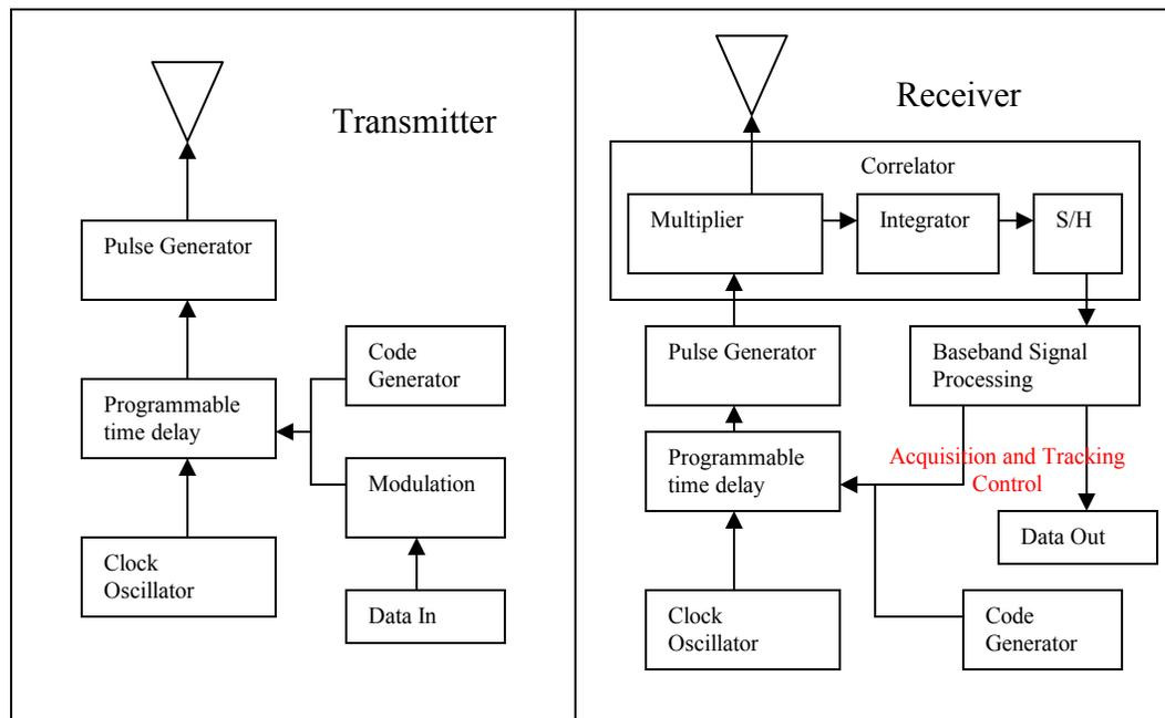
Figure 2. UWB Transmitter-Receiver. Courtesy [2]
