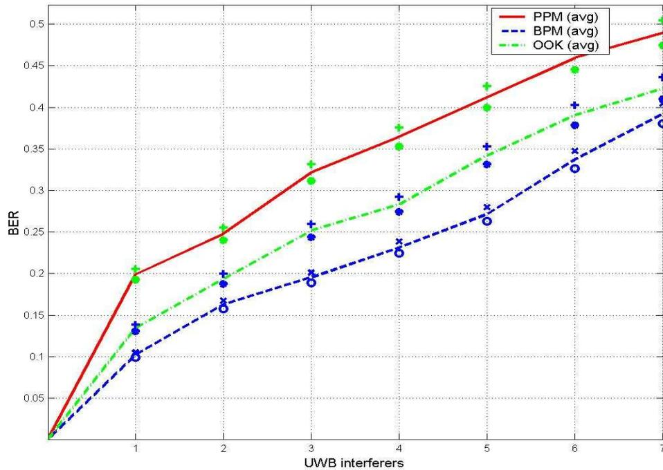
Figure 66. BER vs UWB Interferers (MD, STA to AP – 14 m, 30 Taps)
