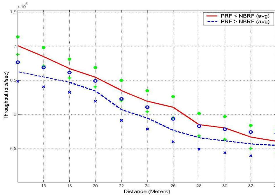
Figure 47. Throughput vs Distance (PRF, 7 UWB Interferers, 30 Taps)
