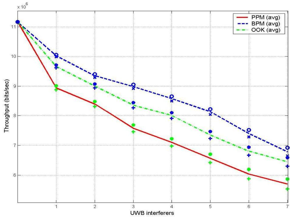
Figure 65. Throughput vs UWB Interferers (MD, STA to AP – 14 m, 30 Taps)
