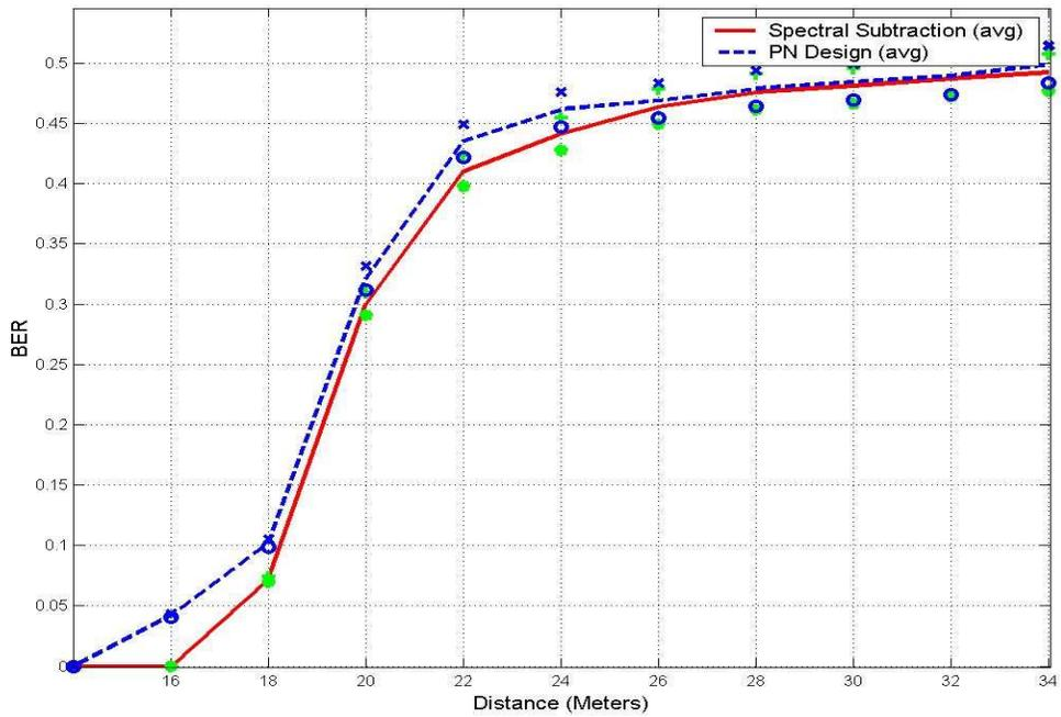
Figure 72. BER vs Distance (MT, 7 UWB Interferers, 30 Taps)
