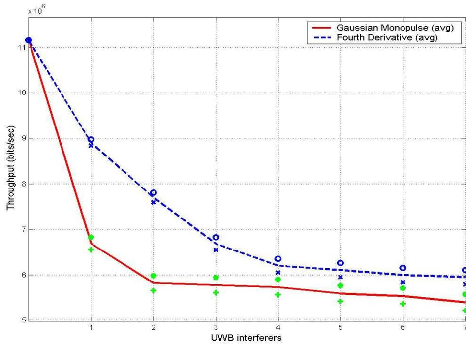
Figure 33. Throughput vs UWB Interferers (PS, STA to AP - 14 m, 30 Taps)
