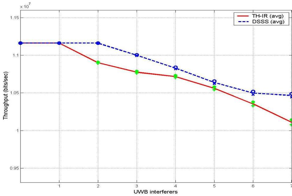
Figure 53. Throughput vs UWB Interferers (ST, STA to AP – 14 m, NM)
