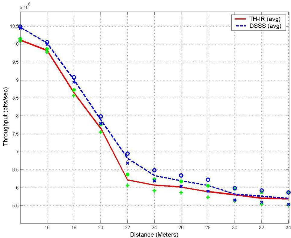
Figure 51. Throughput vs Distance (ST, 7 UWB Interferers, NM)
