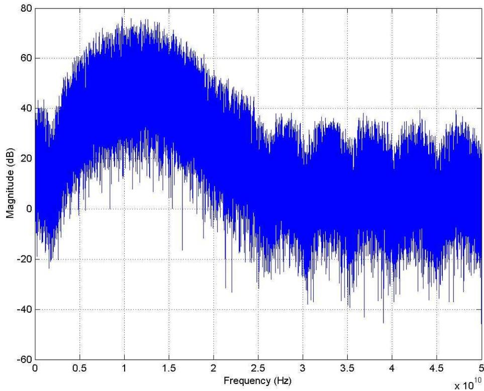
Figure 22. Power Spectrum of DSSS-UWB Signal with 30 Tap Channel
