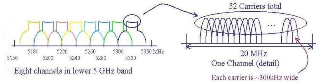
Figure 5. 802.11a Spectrum and Channel Allocation. Courtesy [9]
