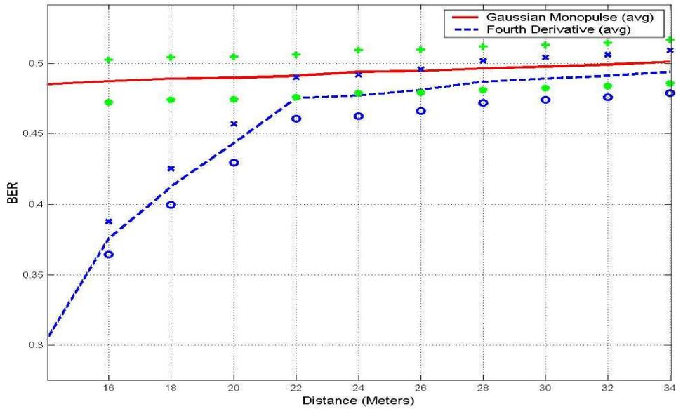
Figure 28. BER vs Distance (PS, 7 UWB Interferers, NM)
