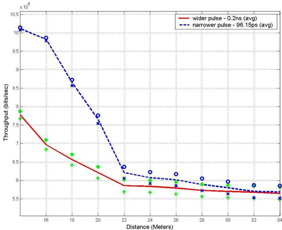
Figure 35. Throughput vs Distance (PW, 7 UWB Interferers, NM)
