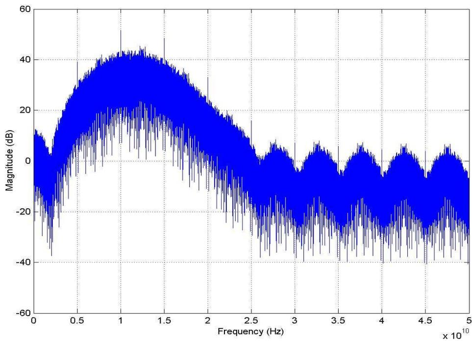
Figure 14. Power Spectrum for UWB Signal with PRF Low (16.66 MHz)
