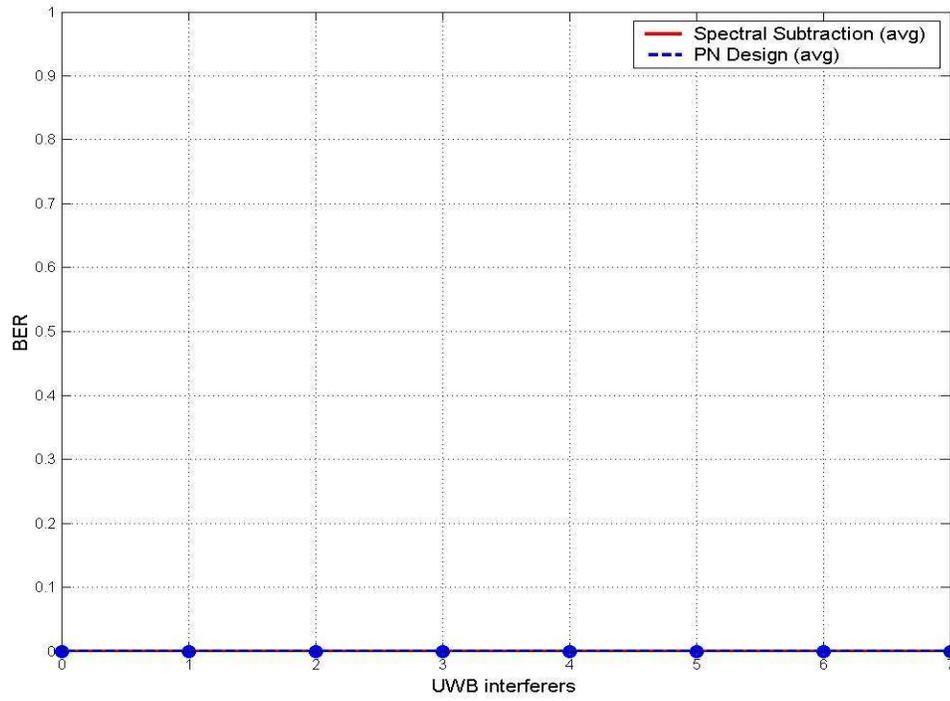
Figure 74. BER vs UWB Interferers (MT, STA to AP – 14 m, 30 Taps)
