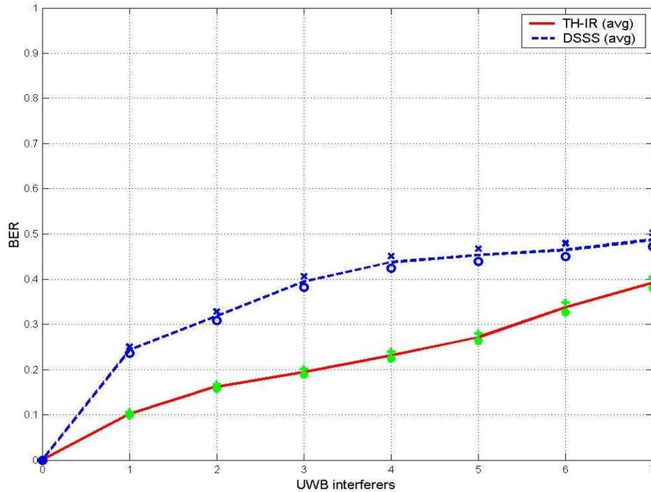
Figure 58. BER vs UWB Interferers (ST, STA to AP – 14 m, 30 Taps)
