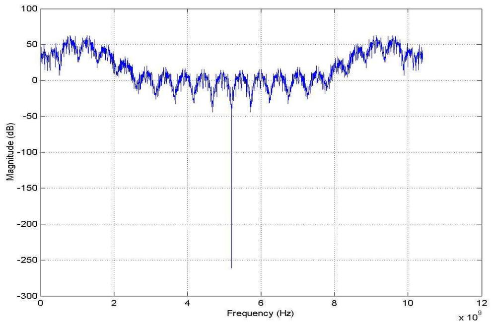
Figure 18. Power Spectrum of UWB signal with Changed Order PN Code
