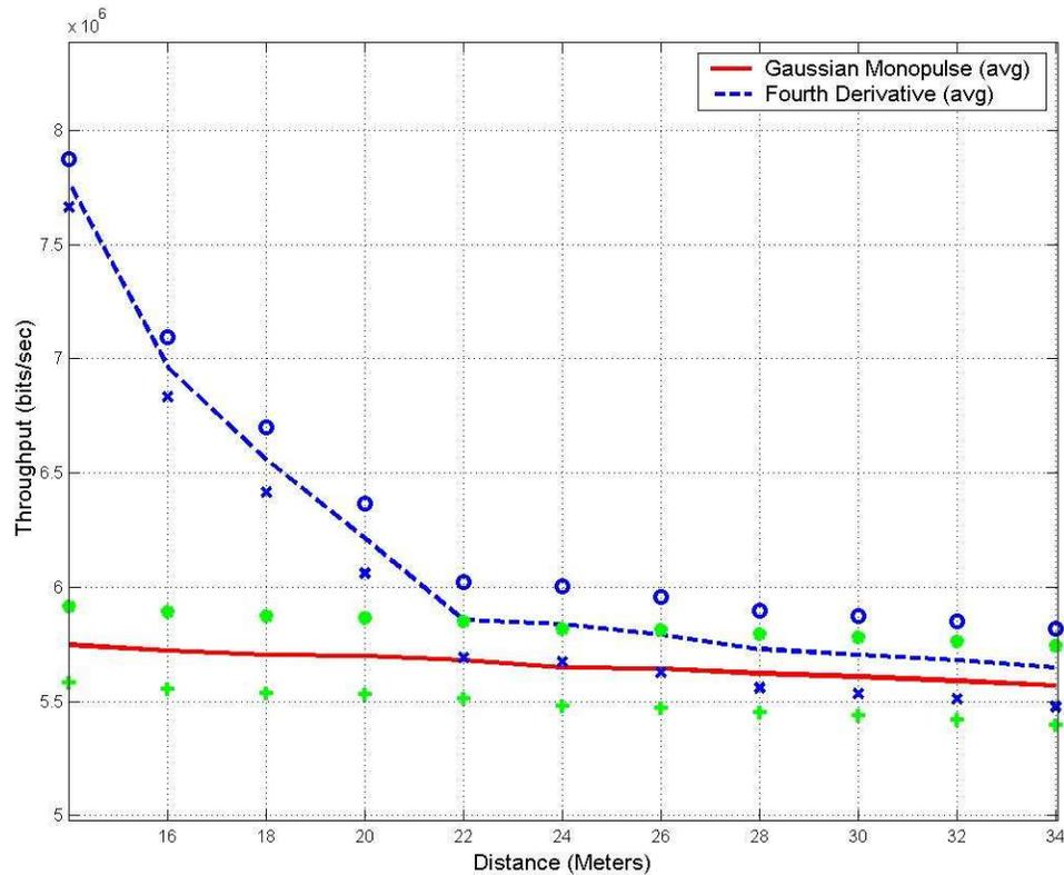
Figure 27. Throughput vs Distance (PS, 7 UWB Interferers, No Multipath (NM))
