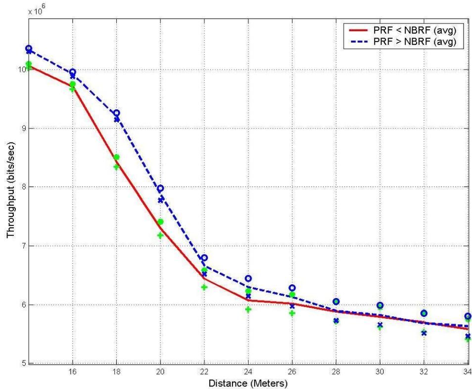
Figure 43. Throughput vs Distance (PRF, 7 UWB Interferers, NM)
