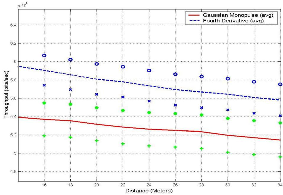
Figure 31. Throughput vs Distance (PS, 7 UWB Interferers, 30 Taps)
