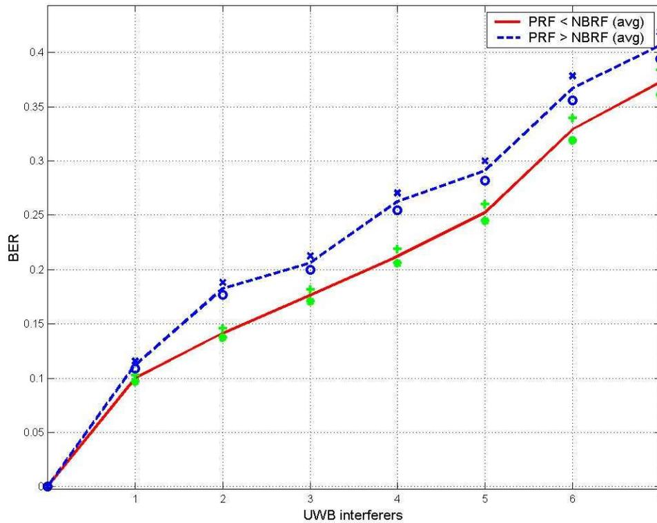
Figure 50. BER vs UWB Interferers (PRF, STA to AP – 14 m, 30 Taps)
