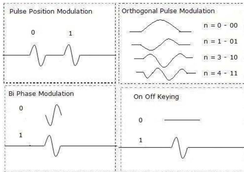
Figure 3. Different Types of Modulation. Courtesy [7]
