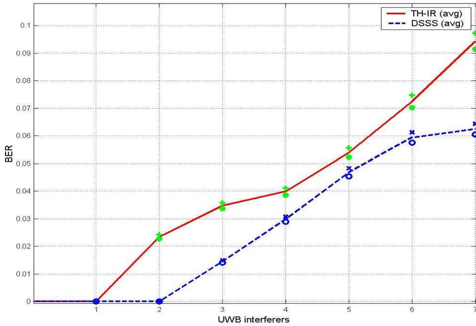
Figure 54. BER vs UWB Interferers (ST, STA to AP – 14 m, NM)
