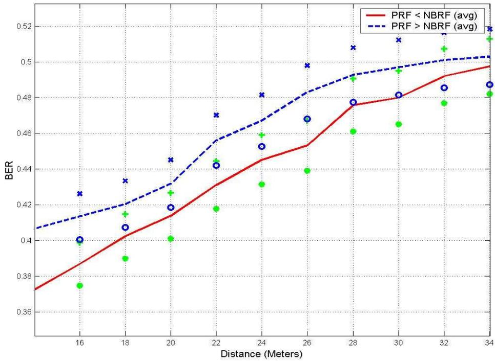
Figure 48. BER vs Distance (PRF, 7 UWB Interferers, 30 Taps)
