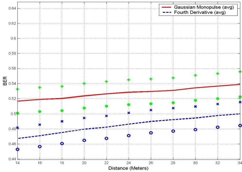
Figure 32. BER vs Distance (PS, 7 UWB Interferers, 30 Taps)
