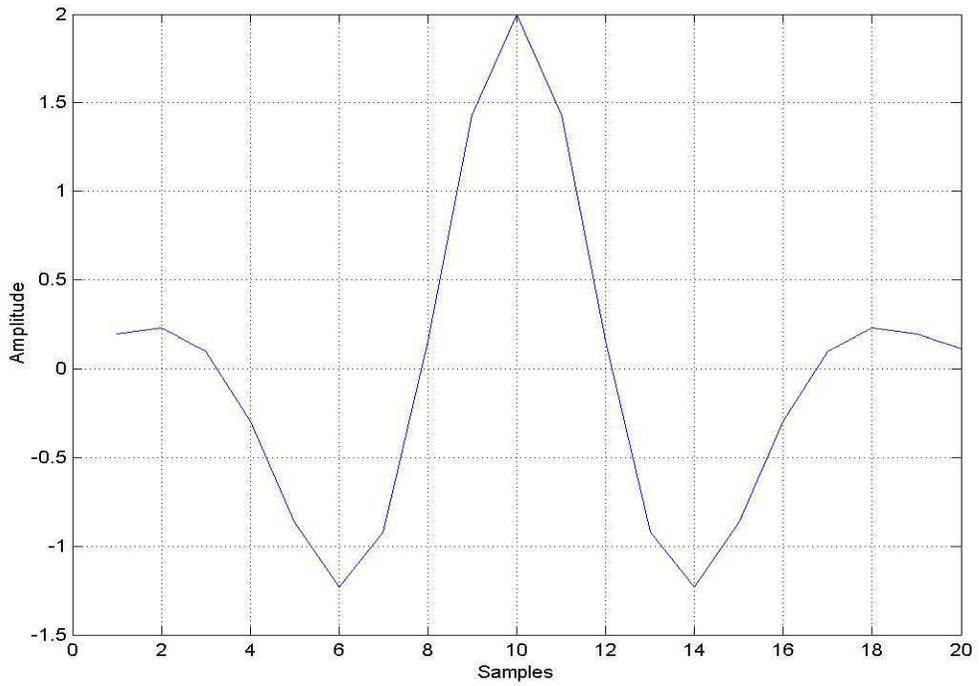
Figure 8. Fourth Derivative of Gaussian Pulse
