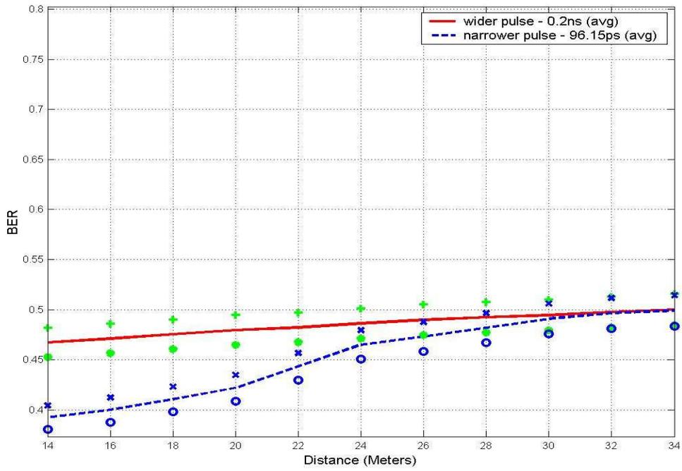
Figure 40. BER vs Distance (PW, 7 UWB Interferers, 30 Taps)
