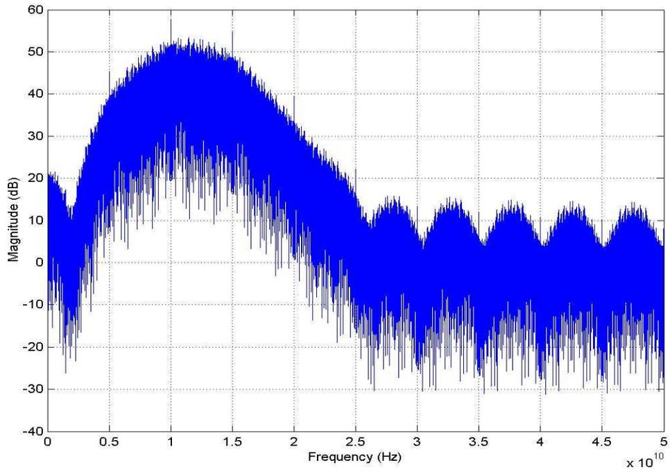
Figure 20. Power Spectrum of UWB Signal with BPM Modulation
