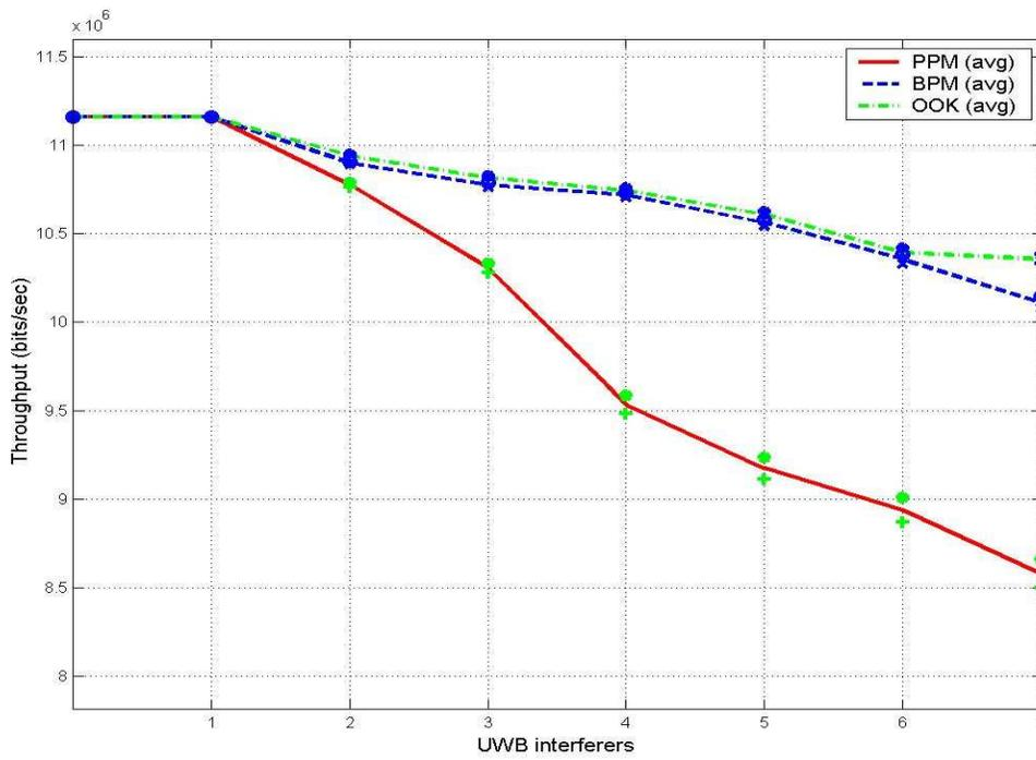
Figure 61. Throughput vs UWB Interferers (MD, STA to AP – 14 m, NM)
