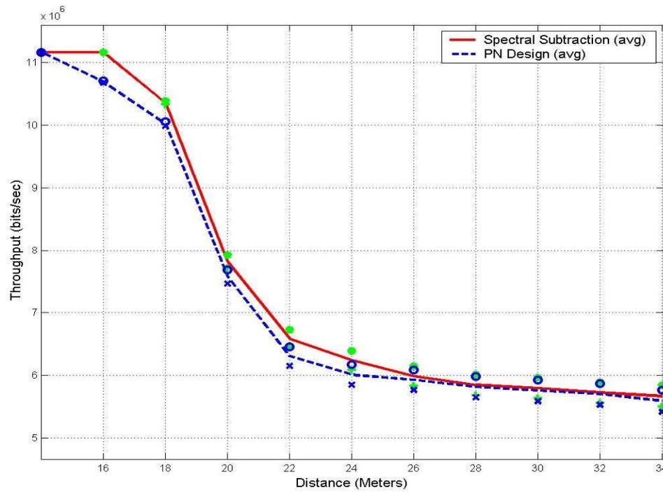
Figure 71. Throughput vs Distance (MT, 7 UWB Interferers, 30 Taps)
