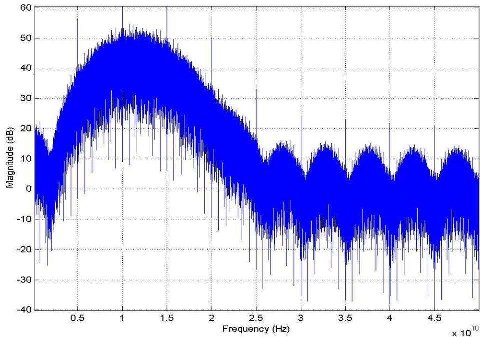
Figure 19. Power Spectrum of UWB Signal with PPM Modulation
