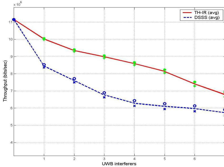
Figure 57. Throughput vs UWB Interferers (ST, STA to AP – 14 m, 30 Taps)
