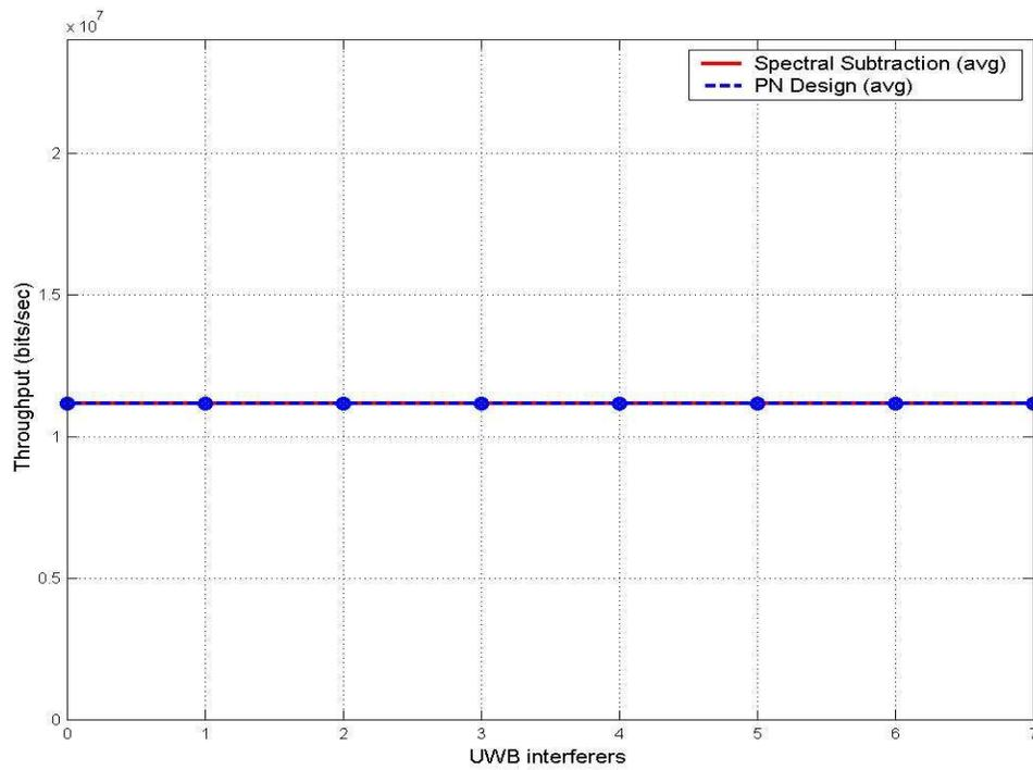
Figure 73. Throughput vs UWB Interferers (MT, STA to AP - 14 m, 30 Taps)
