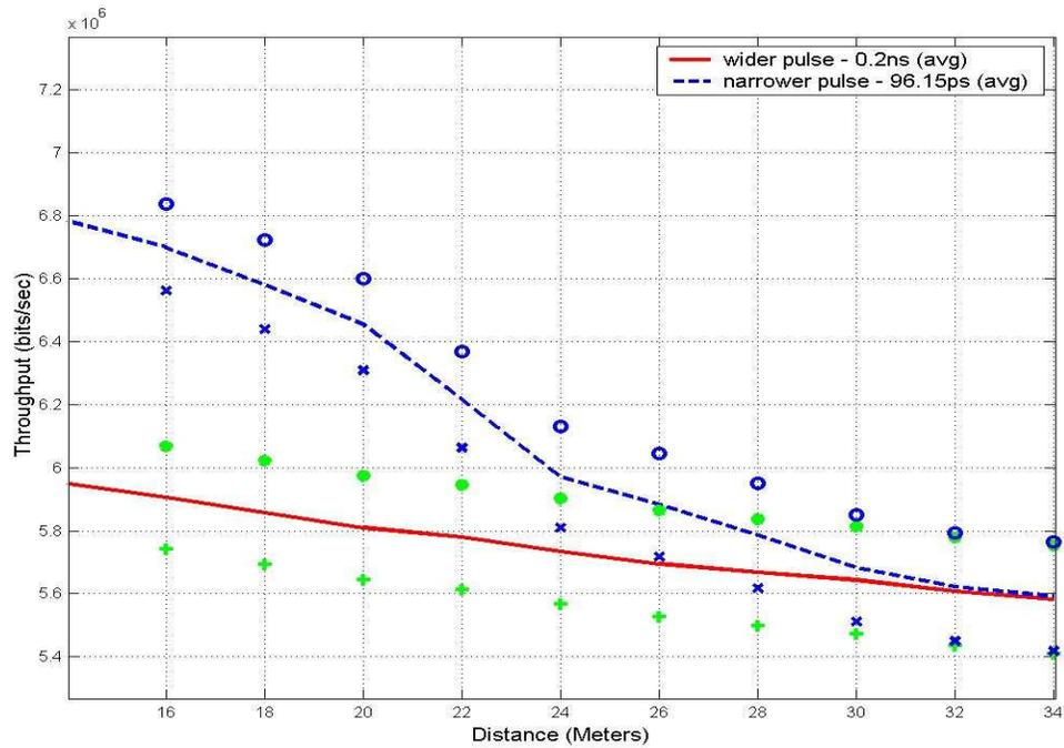
Figure 39. Throughput vs Distance (PW, 7 UWB Interferers, 30 Taps)
