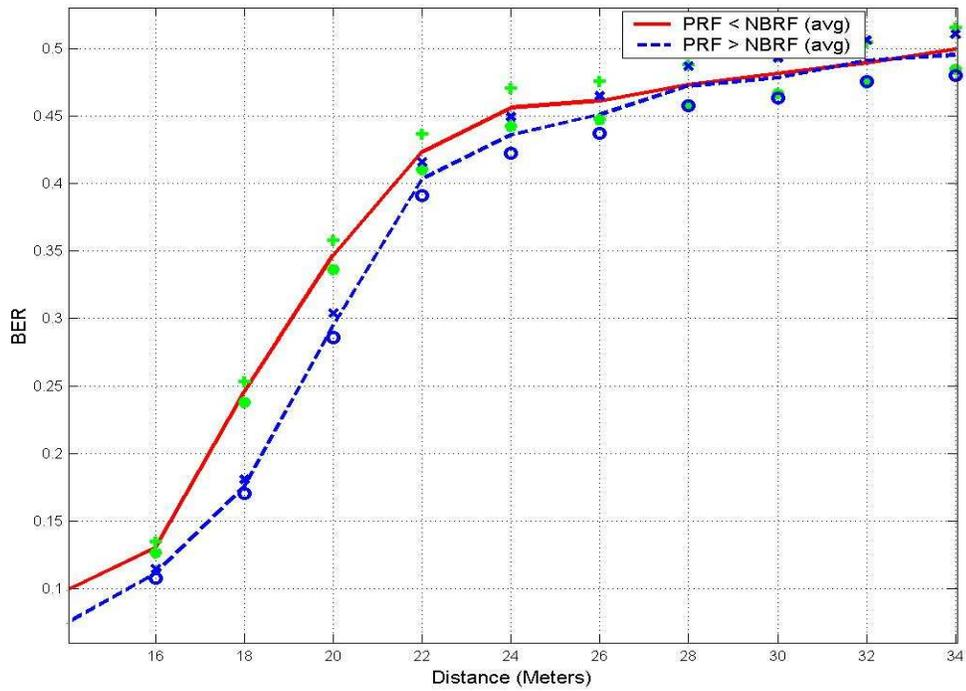
Figure 44. BER vs Distance (PRF, 7 UWB Interferers, NM)
