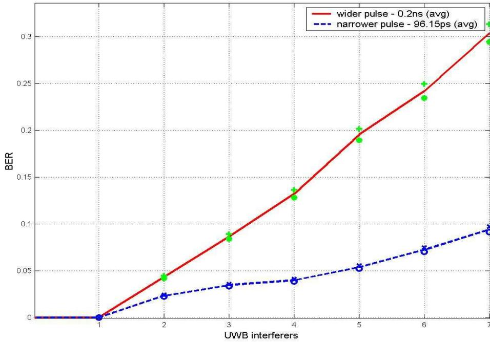
Figure 38. BER vs UWB Interferers (PW, STA to AP – 14 m, NM)
