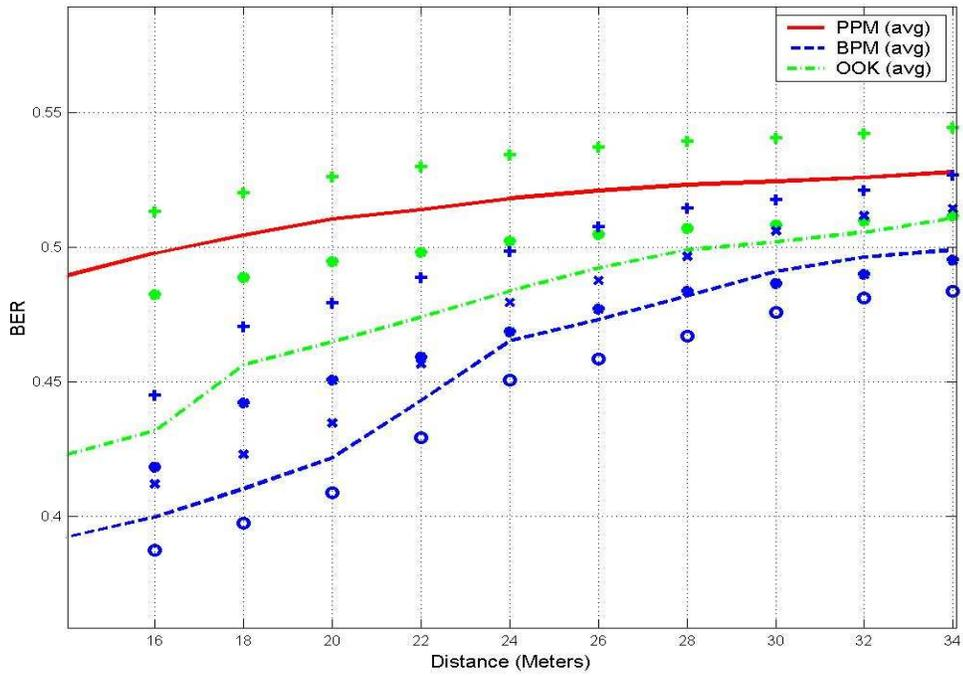
Figure 64. BER vs Distance (MD, 7 UWB Interferers, 30 Taps)
