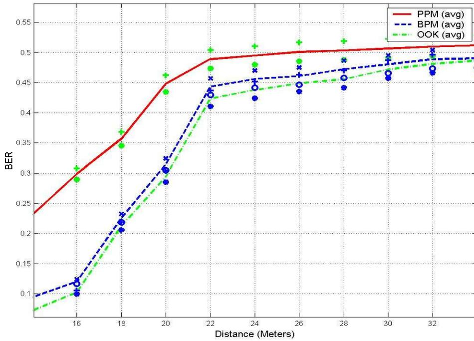
Figure 60. BER vs Distance (MD, 7 UWB Interferers, NM)
