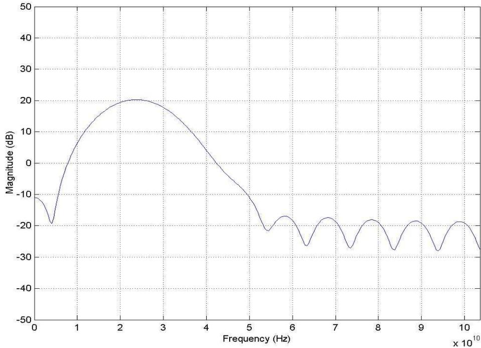
Figure 12. Power Spectrum of Fourth Derivative of Gaussian Pulse (96.15 ps)
