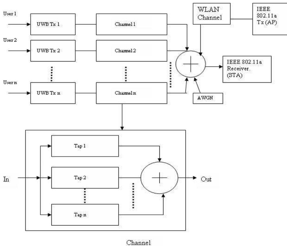
Figure 26. UWB and IEEE 802.11a Coexistence System Model
