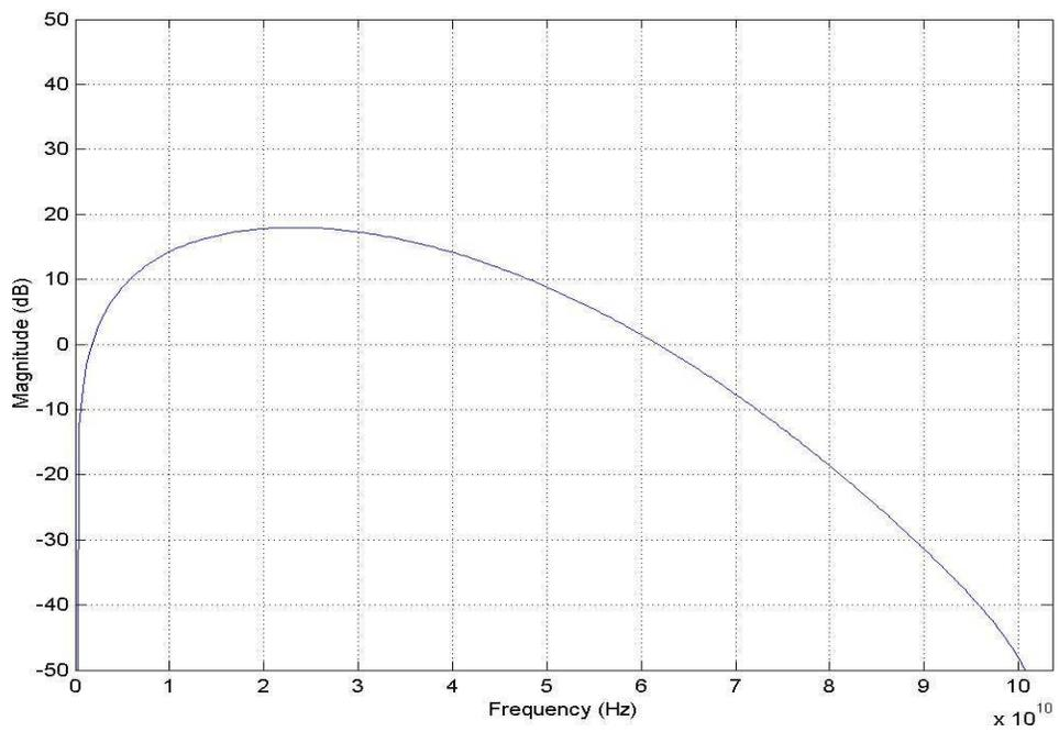
Figure 11. Power Spectrum of Gaussian Monopulse (96.15 ps)
