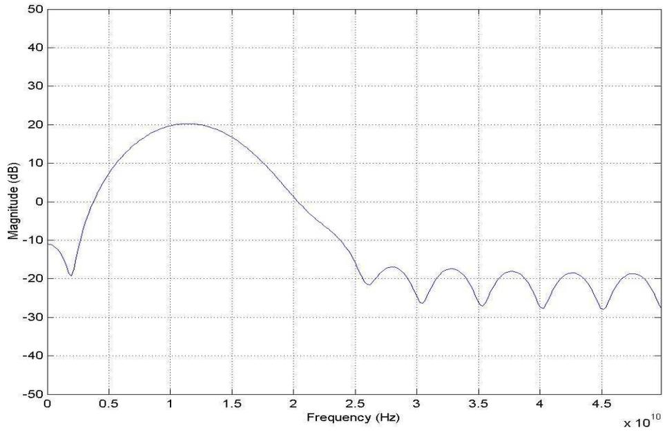
Figure 10. Power Spectrum of Fourth Derivative of Gaussian Pulse (0.2 ns)
