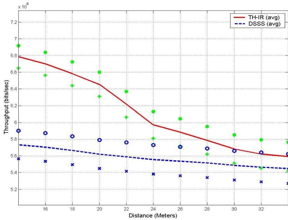
Figure 55. Throughput vs Distance (ST, 7 UWB Interferers, 30 Taps)
