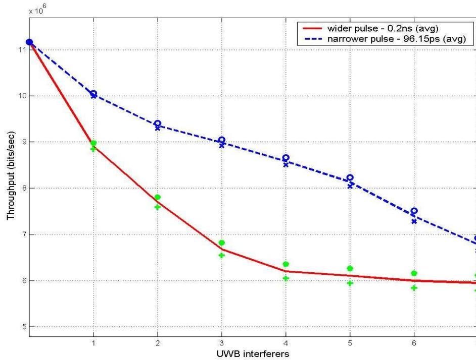
Figure 41. Throughput vs UWB Interferers (PW, STA to AP - 14 m, 30 Taps)
