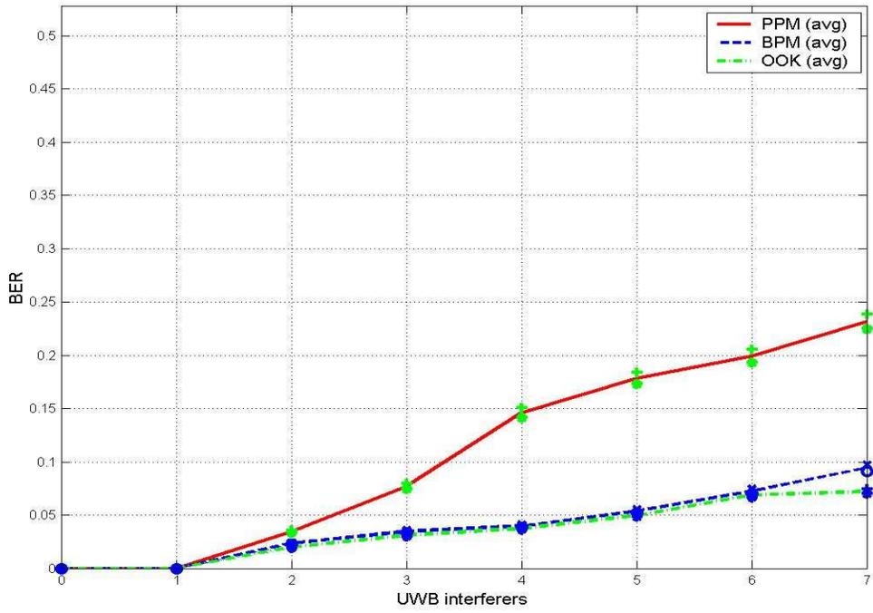
Figure 62. BER vs UWB Interferers (MD, STA to AP – 14 m, NM)
