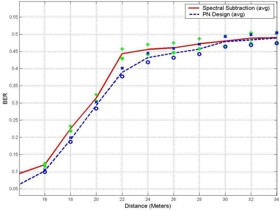
Figure 52. BER vs Distance (ST, 7 UWB Interferers, NM)
