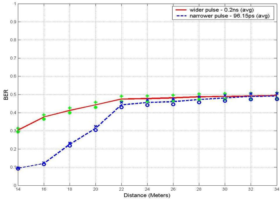
Figure 36. BER vs Distance (PW, 7 UWB Interferers, NM)
