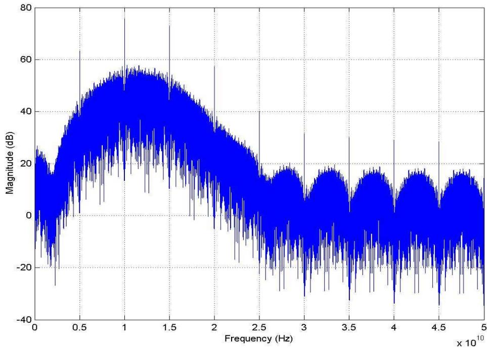
Figure 13. Power Spectrum for UWB Signal with PRF High (100 MHz)
