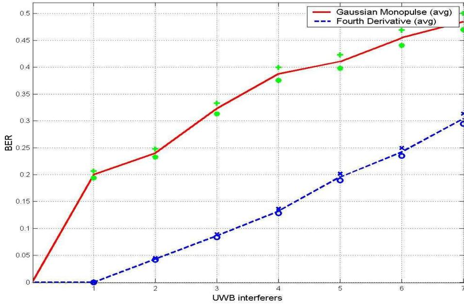
Figure 30. BER vs UWB Interferers (PS, STA to AP – 14 m, NM)
