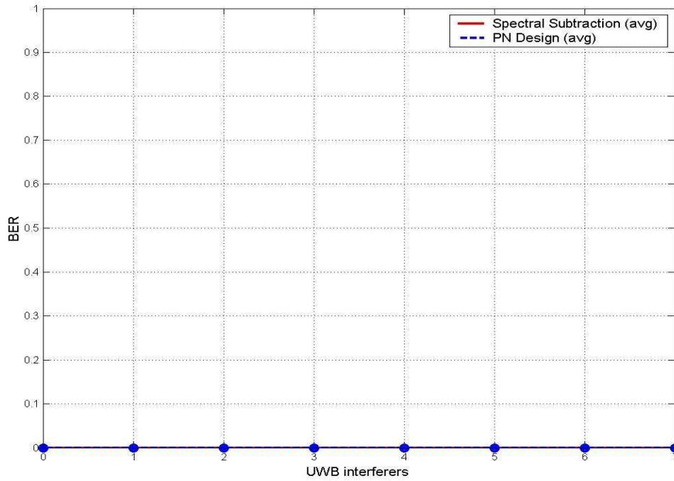
Figure 70. BER vs UWB Interferers (MT, STA to AP – 14 m, NM)
