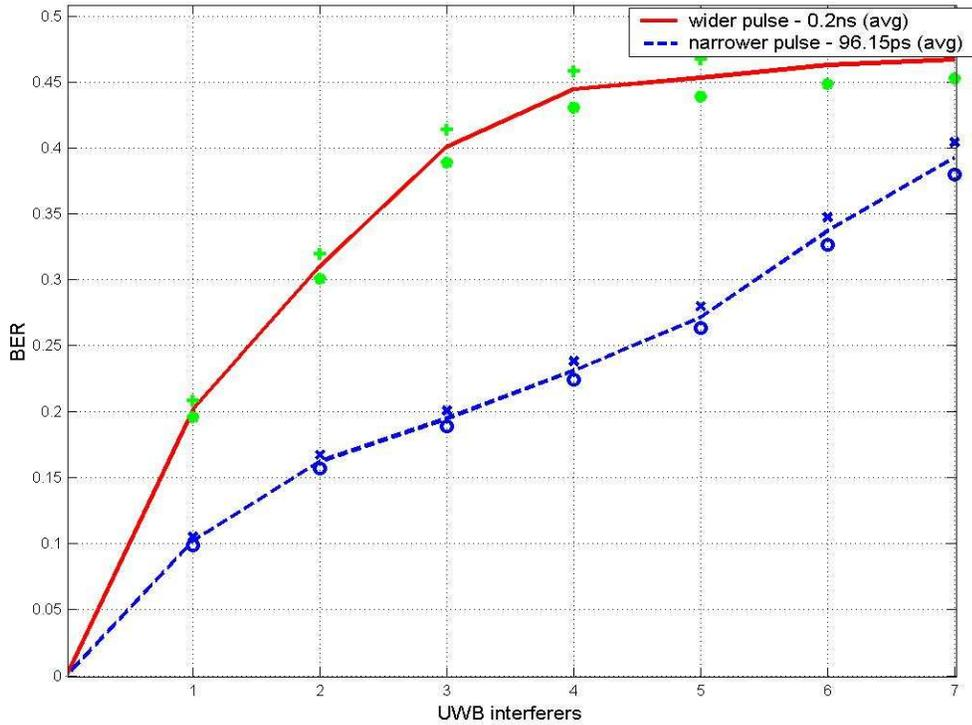
Figure 42. BER vs UWB Interferers (PW, STA to AP – 14 m, 30 Taps)
