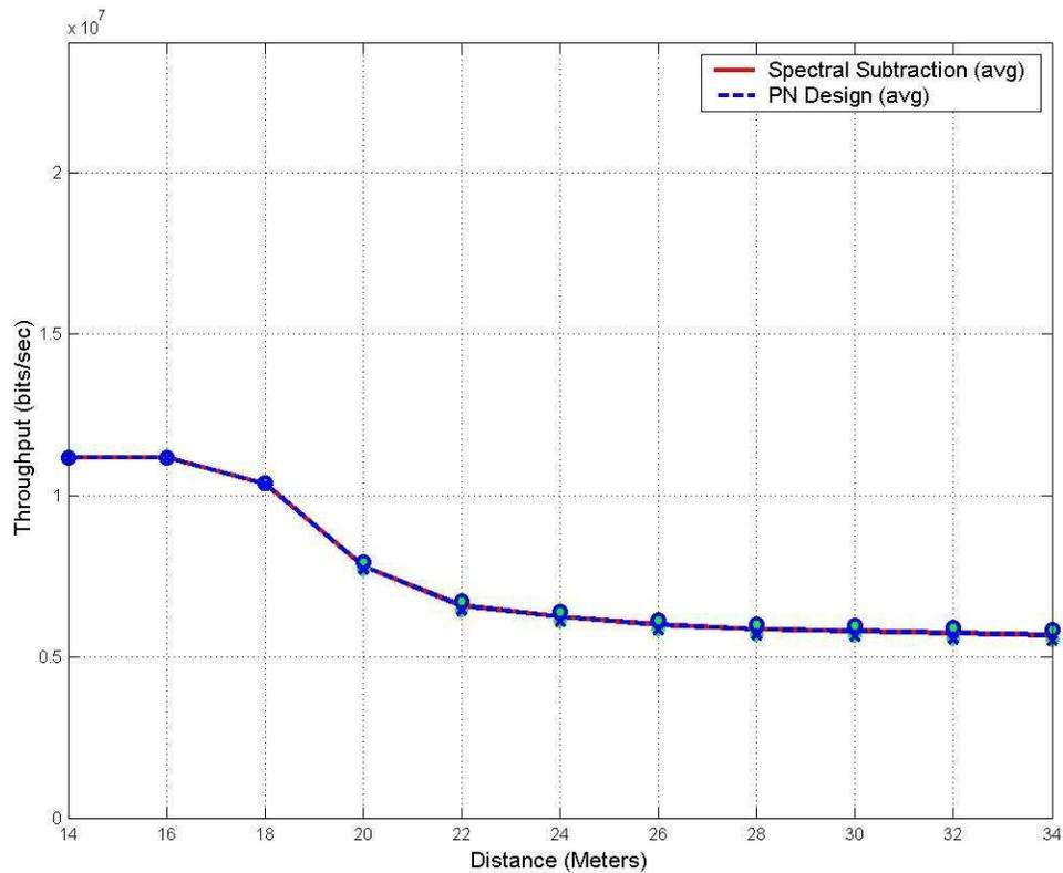
Figure 67. Throughput vs Distance (MT, 7 UWB Interferers, NM)
