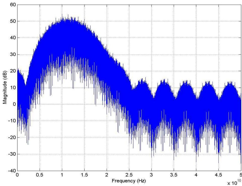
Figure 16. Power Spectrum of TH-IR UWB in a Single Tap Channel
