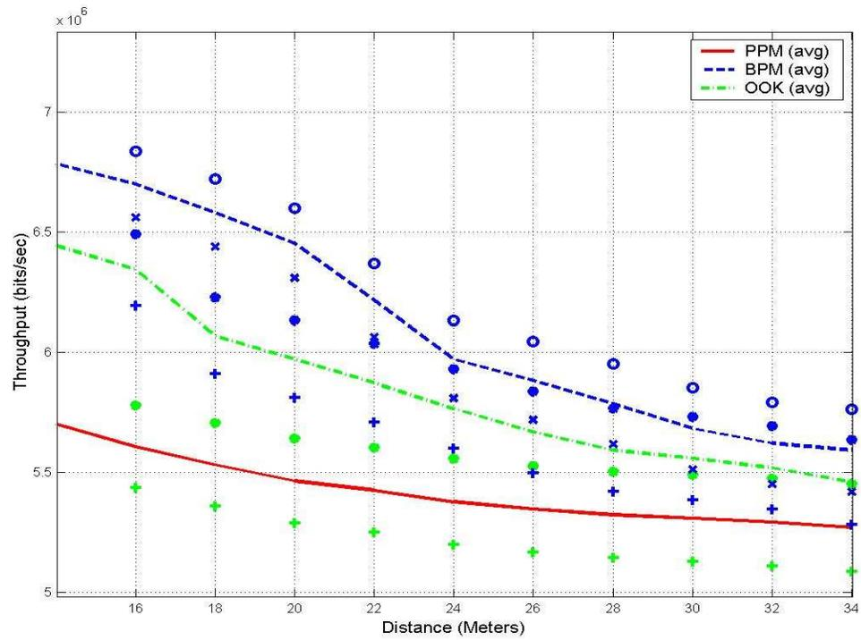
Figure 63. Throughput vs Distance (MD, 7 UWB Interferers, 30 Taps)
