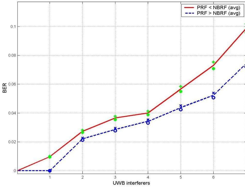
Figure 46. BER vs UWB interferers (PRF, STA to AP – 14 m, NM)
