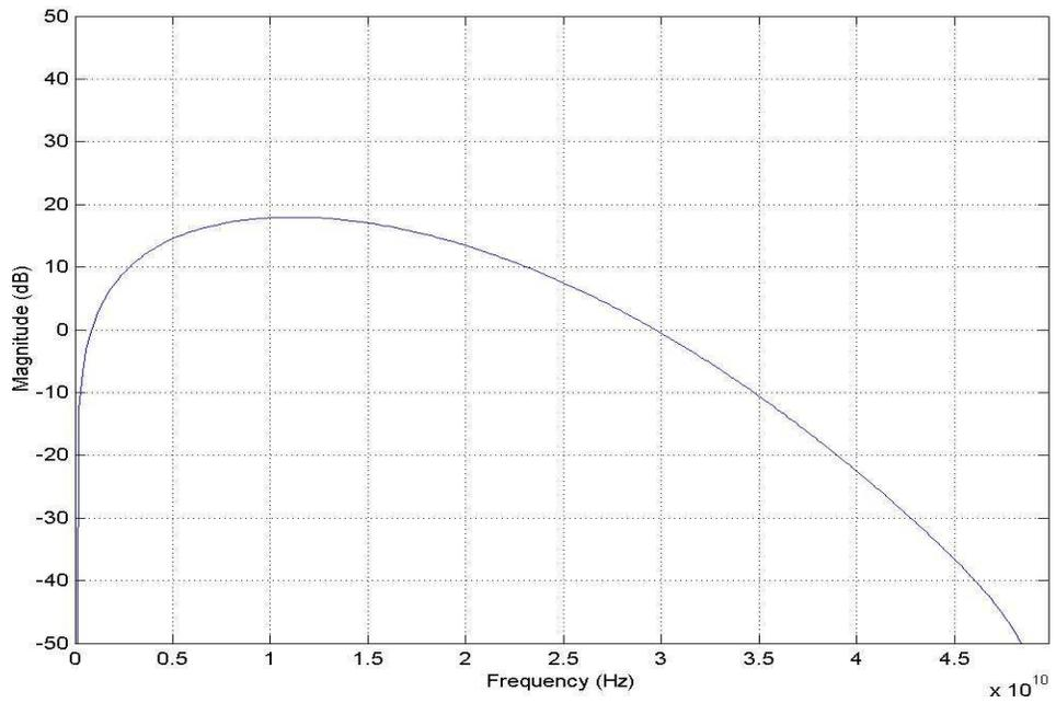
Figure 9. Power Spectrum of Gaussian Monopulse (0.2 ns)
