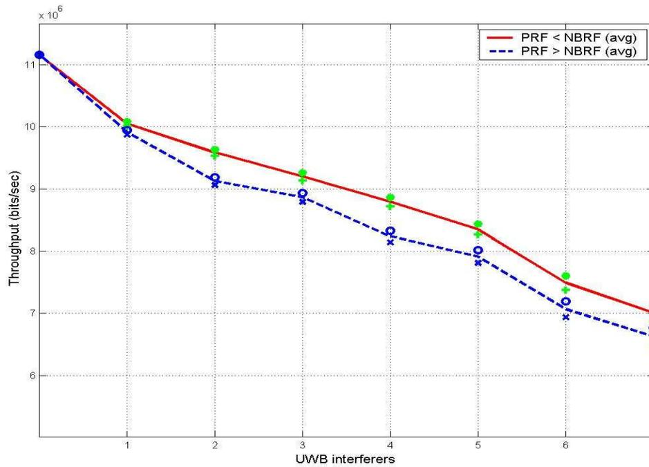
Figure 49. Throughput vs UWB Interferers (PRF, STA to AP – 14 m, 30 Taps)
