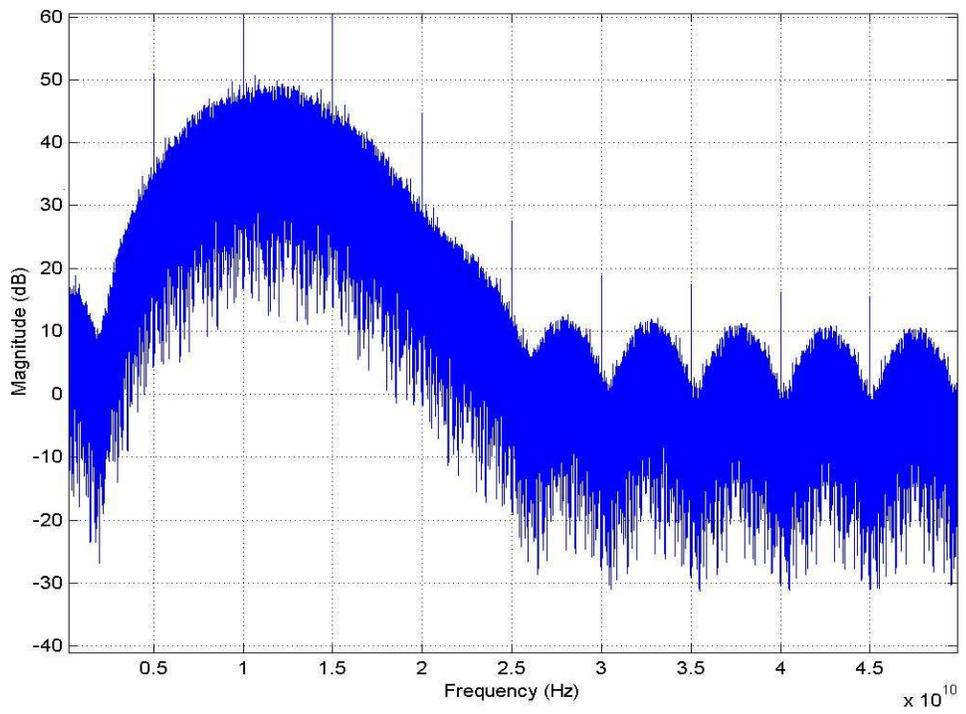
Figure 21. Power Spectrum of UWB Signal with OOK Modulation
