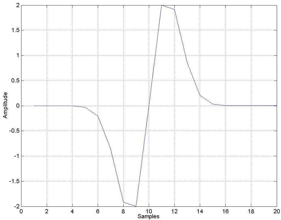
Figure 7. Gaussian Monopulse
