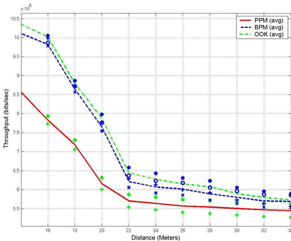
Figure 59. Throughput vs Distance (Modulation (MD), 7 UWB Interferers, NM)
