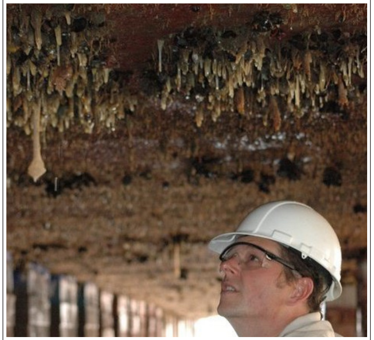
Christopher Brown inspects the bottom of a fouled ship in San Francisco. Copper-containing antifouling hull coatings are a source of copper contamination in marinas and bays. Photo: Smithsonian Environmental Research Center, Marine Invasions Research Lab
