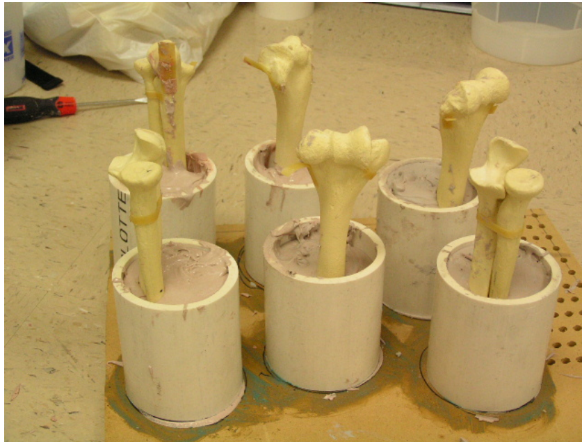
Figure 20: Disarticulated Sawbones with the humerus and forearms potted in PVC tubes with Bondo.
