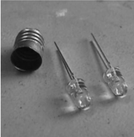
divide the 6.8V lead acid voltage by two, then 3.4V per LED should give a current of about 15 mA. [A gel-cell when fully charged produces about 6.2V, and this gradually ramps down to about 5.8V as the battery is discharged and then falls more rapidly to about 5.4V by which stage the
