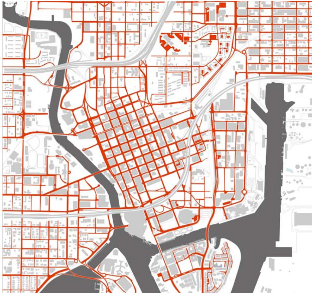
Figure 7.9., Street Grid, shows how Tampa's downtown street grid breaks apart as it collides with the Crosstown Expressway.
