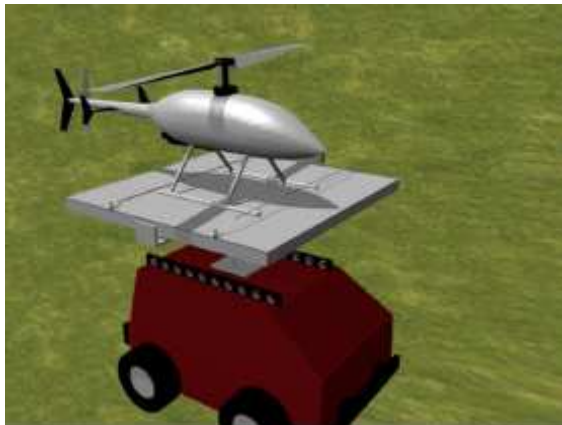
Figure 5-7: A 3D Representation of the Helicopter Landed on the Platform and Secured With a Latching Mechanism.
