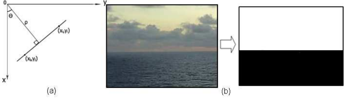
Figure 4.1. Horizon representation. (a) The horizon is represented as a straight line in polar coordinates with parameters \rho and \Theta . (b) Groundtruth for an image. The white color regions corresponds to the sky (above the horizon), black regions correspond to the ocean surface.
