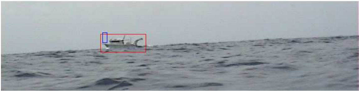
Figure 6.3. Examples of ship detection in video. The picture on the bottom shows an example of failure of detection due to temporal fragmentation of the tracks.
