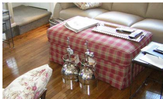
Figure 1. Example of Collection of Indoor Air Samples using Summa® or equivalent canisters
