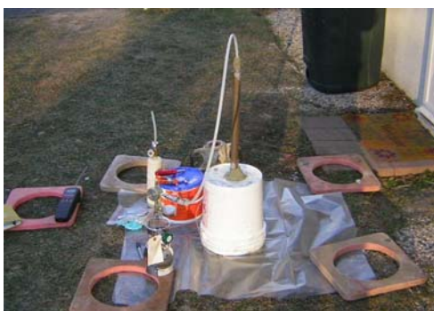
Figure 2. Example of Collection of Soil Vapor Sample from a Temporary Soil Vapor Point using a Summa® or equivalent canister
