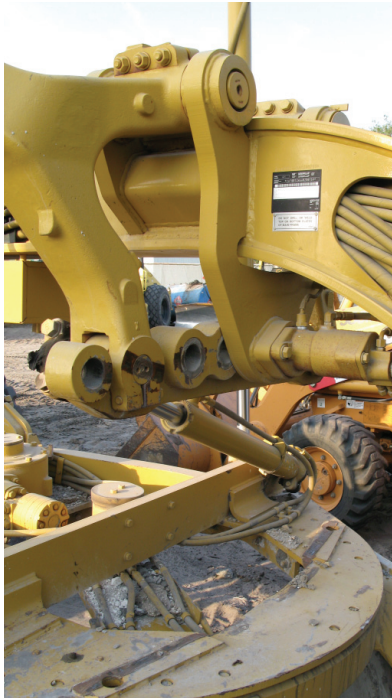
Figure 1.5. Left. Integrated structure and systems delivery on grader
