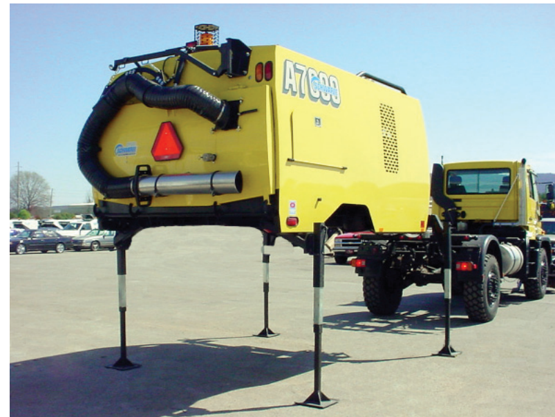
Figure 2.8 Unimog with detachable street sweeper. “Schwarze Industries.” < http://www.schwarze.com/PressReleases/A7UNIMOG.html >.
