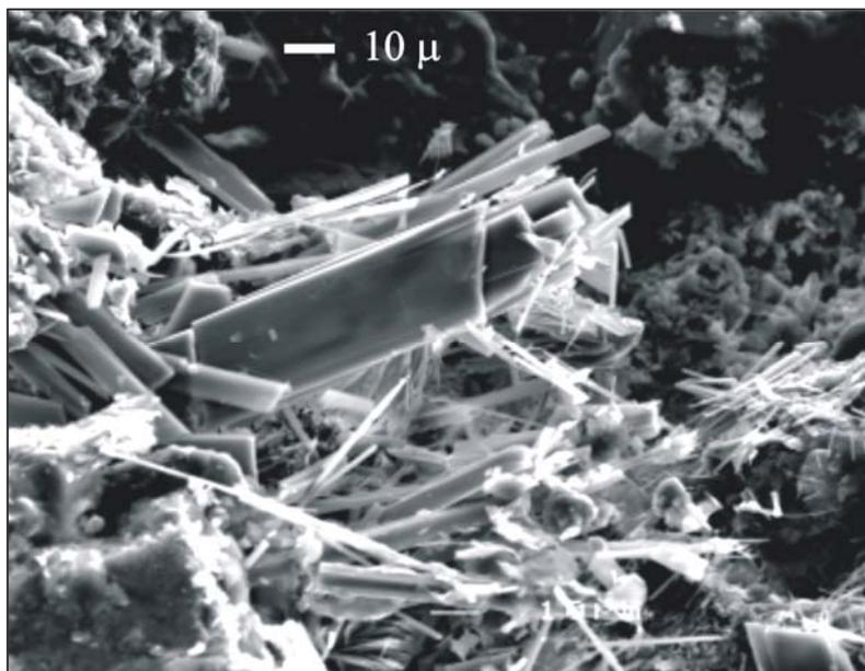
Fig. 1. Scattered serpierite crystals (SEM image).
