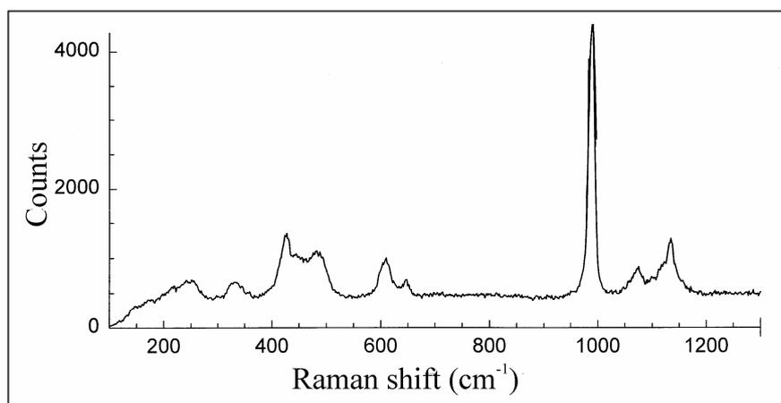
Fig. 4. Raman spectrum of serpierite.
