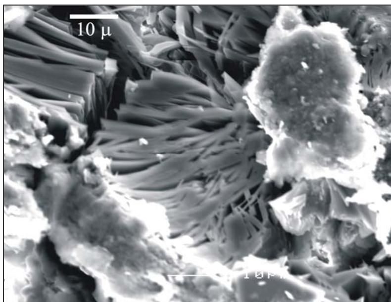
Fig. 2. Packed serpierite crystals (SEM image).
