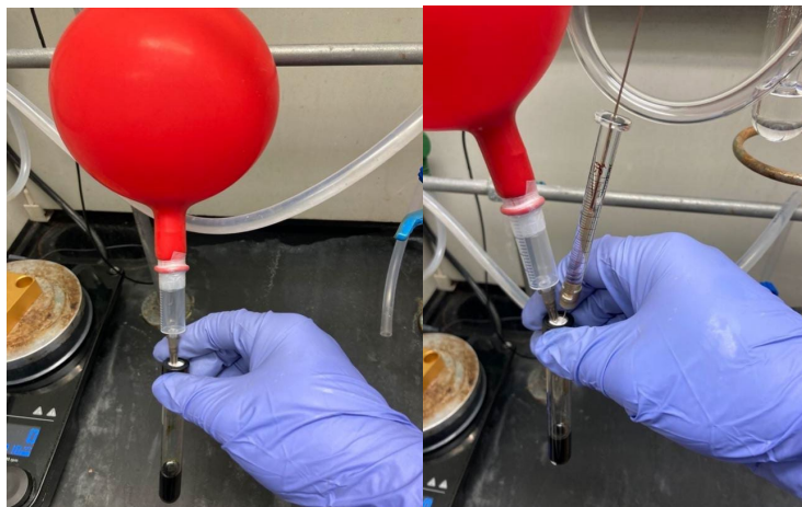
Figure S3: Graphical procedure for Co-catalyzed hydroamination (part A). Left: Addition of catalyst, alkene, and solvent to reaction vial. Right: Addition of diazirine 2 to reaction mixture.
