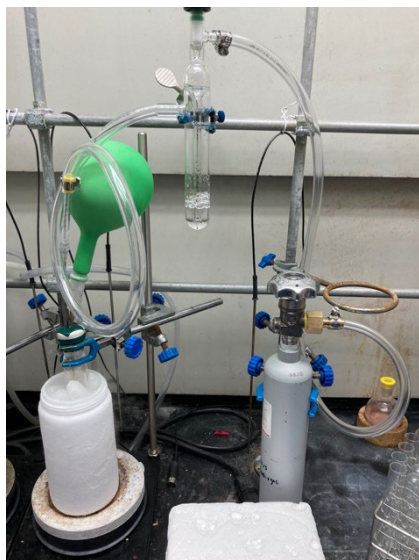
Figure S10: Bubbling ^{15}\text{NH}_3 gas into the \text{PPh}_3\text{Br}_2 suspension with oil bubbler as a flowmeter.
