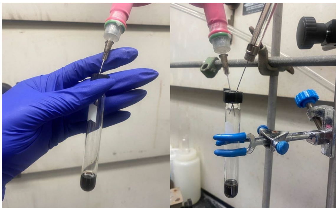
Figure S6: Graphical procedure for Mn-catalyzed hydroamination (part A). Left: Addition of catalyst, alkene, and solvent to reaction vial. Right: Addition of diazirine 2 to reaction mixture.
