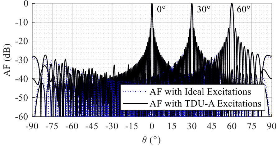
Figure 2.16 Normalized array factor of 128 element linear PAA at  $f = 30$  GHz when it employs the optimum TDU architecture (TDU-A) excitations shown in Fig. 2.13 and ideal excitations.
