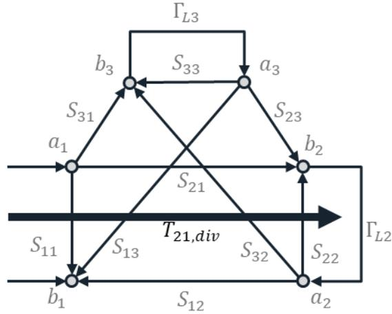
Figure 3.6 Signal flow graph representation of Fig. 3.5 when ports 2 and 3 are terminated with loads.
