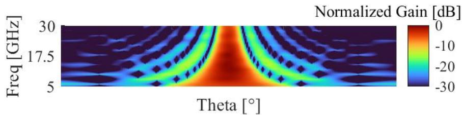
Figure 3.18 Normalized array pattern vs. scan angle and frequency for the TDU-A defined in Fig. 3.12 from model when including delay error steered to  $0^\circ$ .
