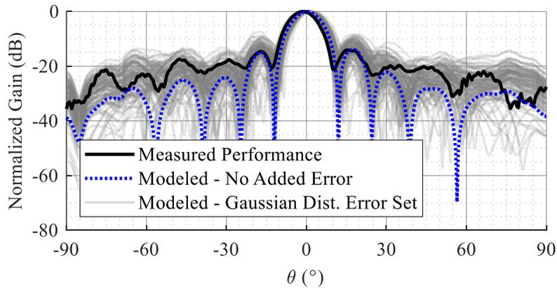
Figure 3.26 Comparison of 18 GHz measurement (bold plots) vs 100 iterations of modeled performance (light gray plots) within the family of expected delay errors in the RF-fanout steered to 0°.
