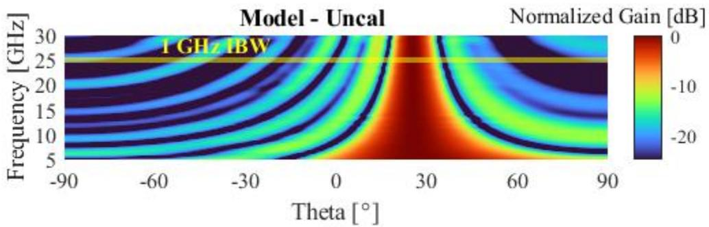
Figure 4.2 Array factor vs frequency of a 16 element array with uncalibrated EM TDU-A simulated excitations.
