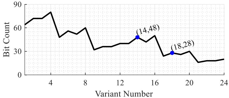
Figure 2.6 TDU bit count vs variant number of the 8 element PAA. Data points correspond to variants shown in Figs. 2.3 and 2.4.
