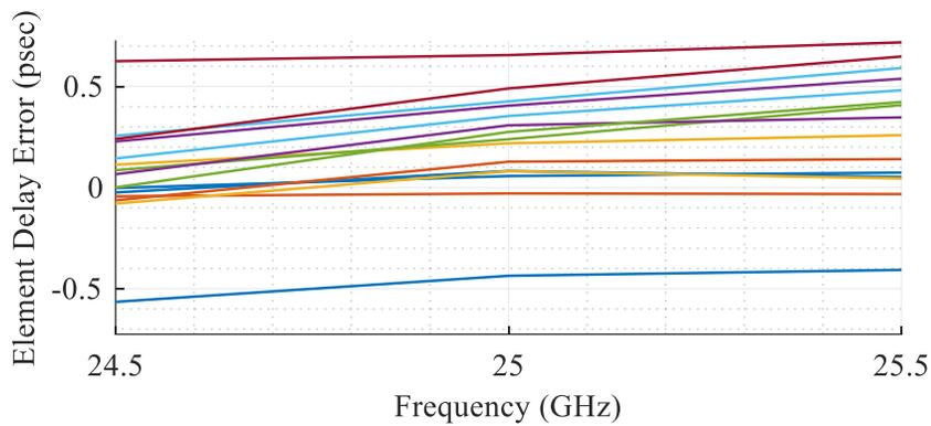
Figure 4.7 Distribution of delay error of the EM simulated TDU-A excitations for each element when compared to an ideal excitation after calibration at 25 GHz zoomed into the calibration window.
