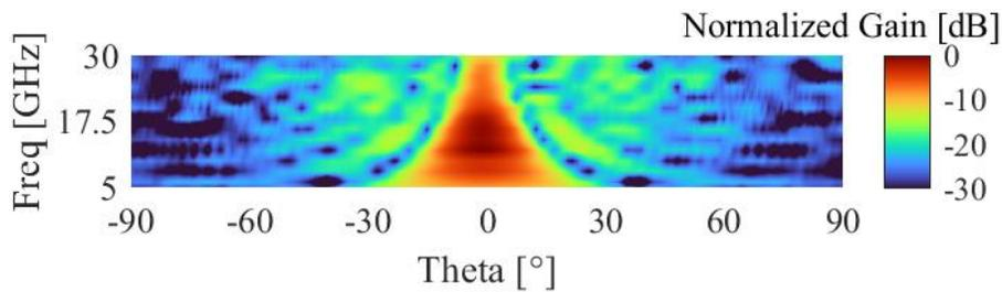
Figure 3.19 Normalized array pattern vs. scan angle and frequency for the TDU-A defined in Fig. 3.12 measured patterns from hardware steering to  $0^\circ$ .
