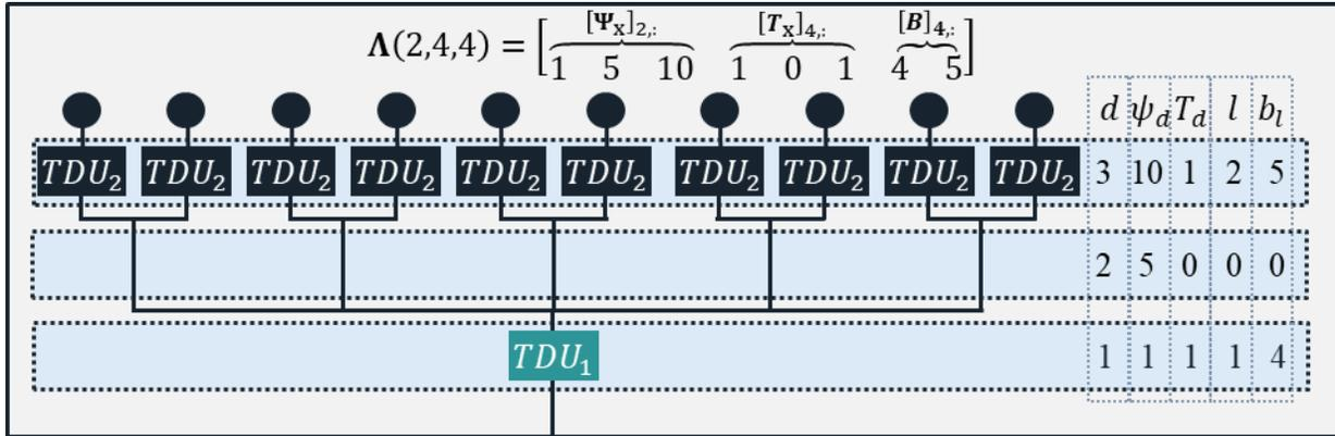
Figure 5.5 Architecture variant examples for a  $D_x = 3$  division level 10 element PAA with a 5-way divider followed by a 2-way divider with a 4 bit TDU layer in  $d = 1$  and 5 bit TDU layer in  $d = 3$  with no TDUs in  $d = 2$ .
