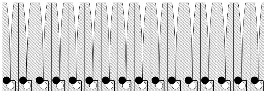
Figure 3.14 A 16 element array model with two terminated elements on both sides to reduce edge effects totaling 20 elements.
