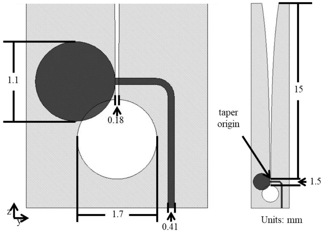
Figure 3.13 Antenna element geometry.
