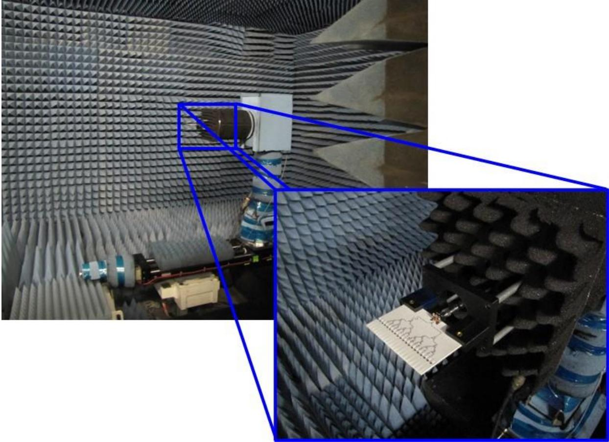
Figure 3.16 16 element PAA with feed network implemented for  $0^\circ$  beam steering during measurement inside an anechoic chamber.
