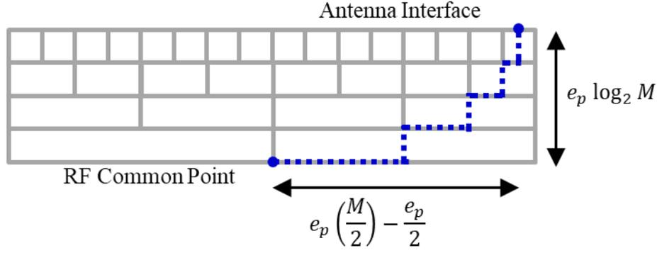
Figure 3.11 Illustration of the allowable area for the corporate feed network implementation pursued for the  $M=16$  element PAA. The dashed path represents the reference distance to the antenna interface.
