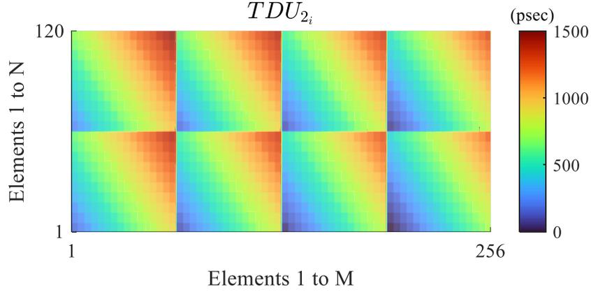
Figure A.4 TDU settings for layer 2 of the architecture in Fig. 5.11 for a  $256 \times 120$  element PAA steered to  $\theta_{zx} = 60^\circ$  and  $\theta_{zy} = 30^\circ$ .
