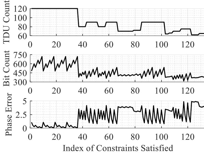
Figure 5.10 TDU count, bit count, and RMS phase error vs index of variants that satisfy the constraints for the  $10 \times 6$  PAA example.
