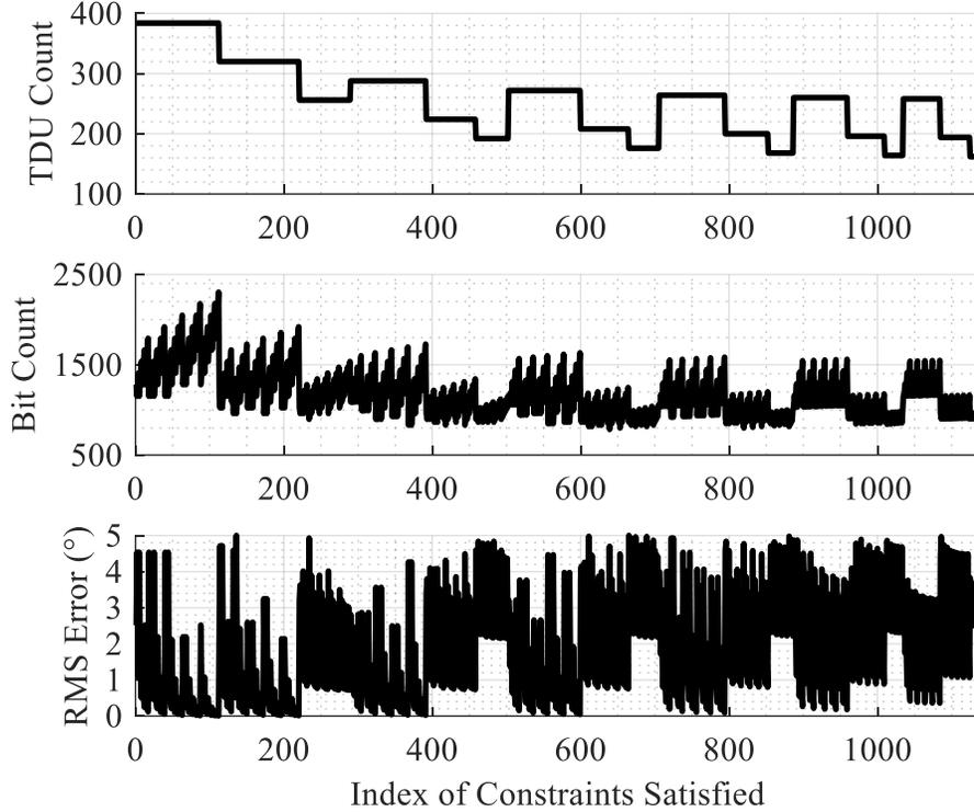
Figure 2.12 TDU count, bit count, and RMS phase error across variants of the 128 element PAA that meet the performance constraints.
