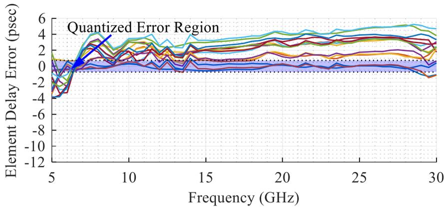
Figure 4.8 Distribution of delay error of the EM simulated TDU-A excitations for each element when compared to an ideal excitation after calibration at 6.5 GHz with a 100 MHz IBW.
