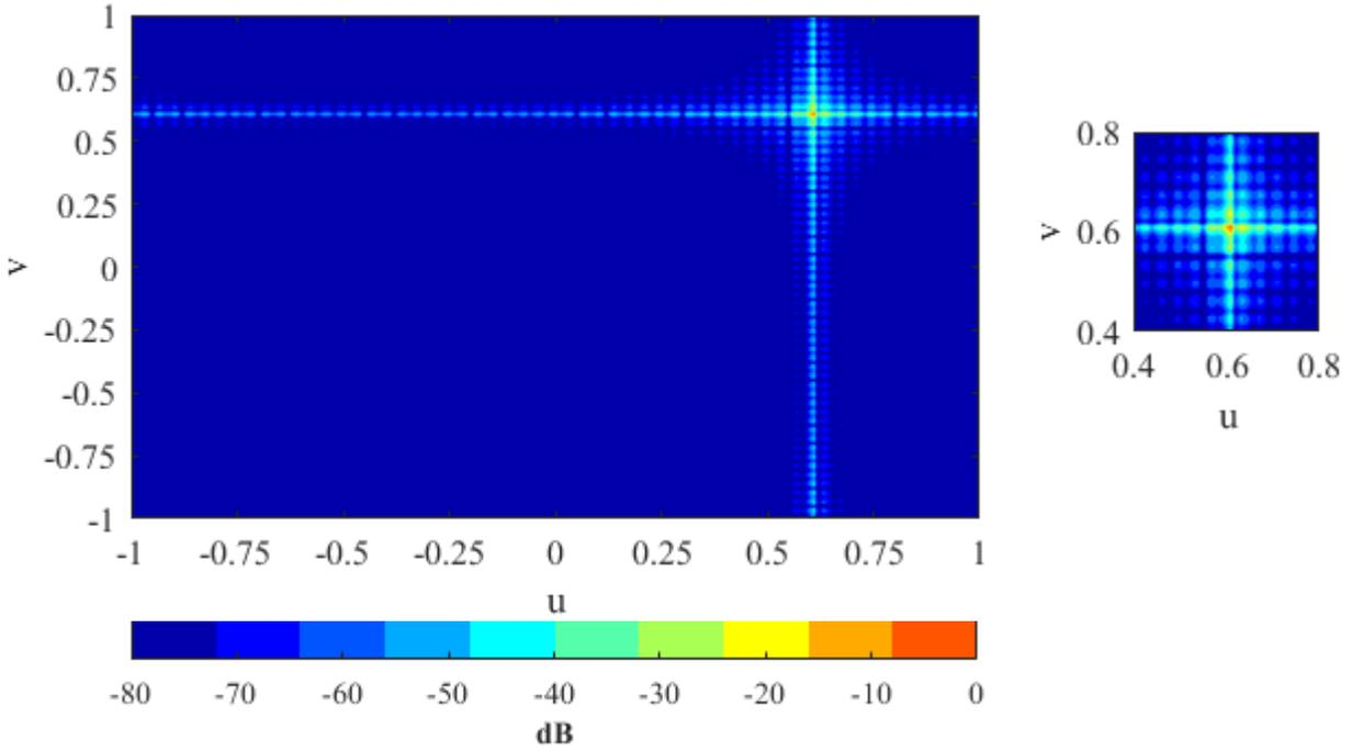
Figure 2.18 Array factor of  $256 \times 256$  PAA when beam is scanned to  $\theta = 60^\circ, \phi = 45^\circ$  using phase delays that are ideal.
