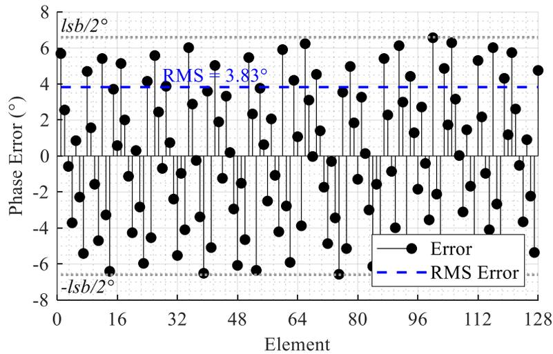
Figure 2.14 Phase error at each element of the 128 element PAA which is bounded by half the lsb at  $TDU_3$ . The phase error exhibits an RMS value of  $3.83^\circ$  at  $f_{max} = 30$  GHz and  $\theta_{scan} = 60^\circ$ .
