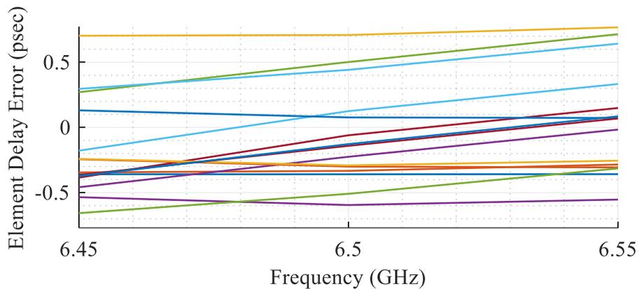
Figure 4.9 Distribution of delay error of the EM simulated TDU-A excitations for each element when compared to an ideal excitation after calibration at 6.5 GHz zoomed into the calibration window.
