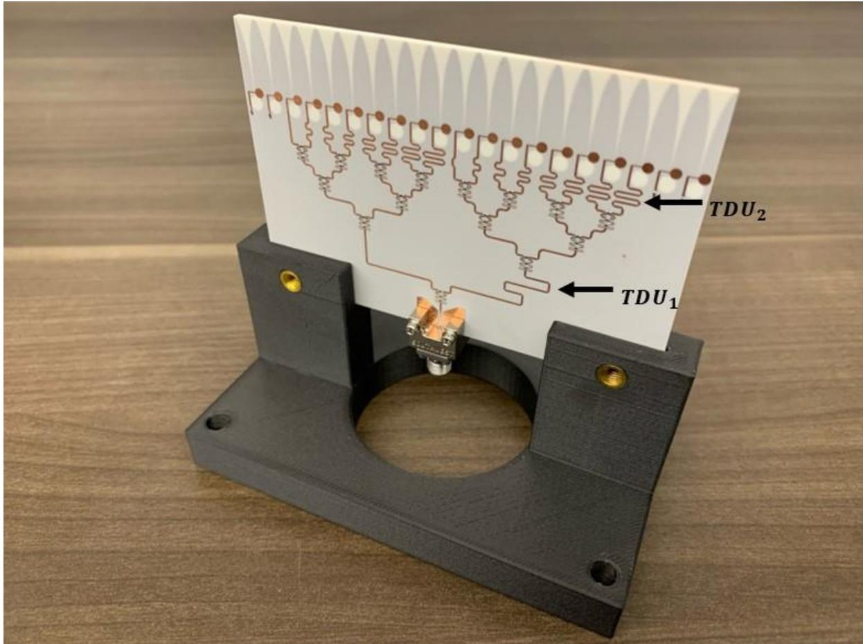
Figure 3.15 Fabricated 16 element linear PAA with feed network implemented for 50° beam steering.
