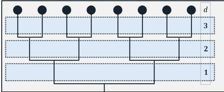
Figure 2.2 Three division level RF-fanout of an 8 element linear array, where TDU bits can potentially be placed in each division level with different combinations.
