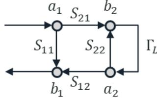
Figure 3.9 Signal flow graph representation of Fig. 3.8 when port 2 is terminated with a load.
