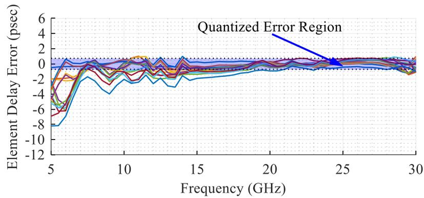
Figure 4.6 Distribution of delay error of the EM simulated TDU-A excitations for each element when compared to an ideal excitation after calibration at 25 GHz with a 1 GHz IBW.
