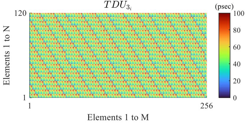
Figure A.6 TDU settings for layer 3 of the architecture in Fig. 5.11 for a  $256 \times 120$  element PAA steered to  $\theta_{zx} = 60^\circ$  and  $\theta_{zy} = 30^\circ$ .
