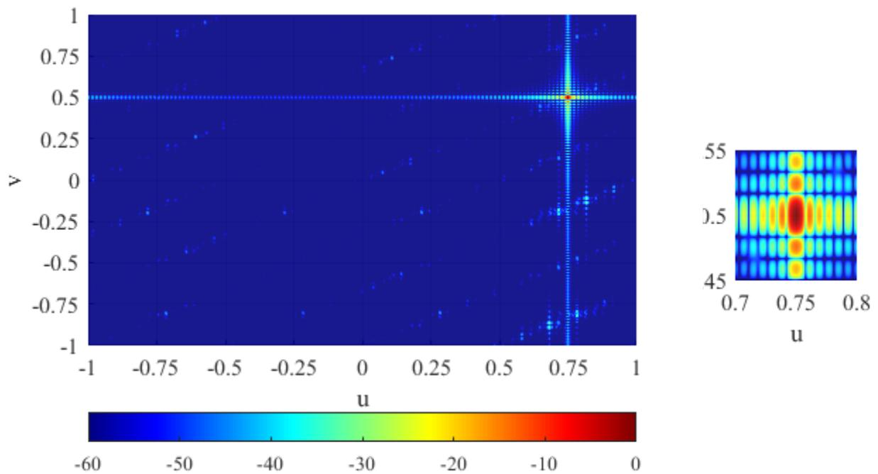
Figure 5.14 AF of  $256 \times 120$  PAA scanned to  $\theta_{zx_{max}} = 60^\circ$  and  $\theta_{zy_{max}} = 30^\circ$  with excitations that are generated by the TDU architecture in Fig. 5.11.
