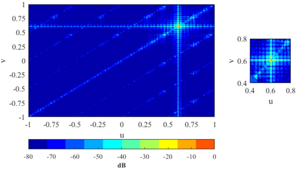
Figure 2.19 Array factor of  $256 \times 256$  PAA when beam is scanned to  $\theta = 60^\circ, \phi = 45^\circ$  using phase delays that are generated by the TDU architecture in Fig. 2.17.
