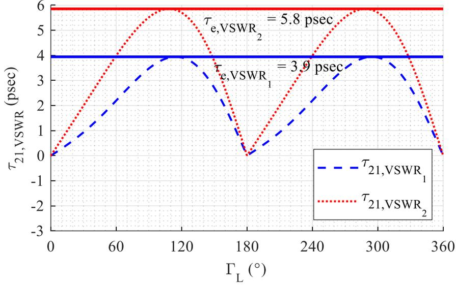
Figure 3.10 Time delay variation of TDU at 5 GHz when terminated with  $\Gamma_L = S_{11}^D = 0.316 e^{-j\theta_{RL}}$  (VSWR<sub>1</sub>) and  $\Gamma_L = S_{11}^{ANT} = 0.5 e^{-j\theta_{ANT}}$  (VSWR<sub>2</sub>)
