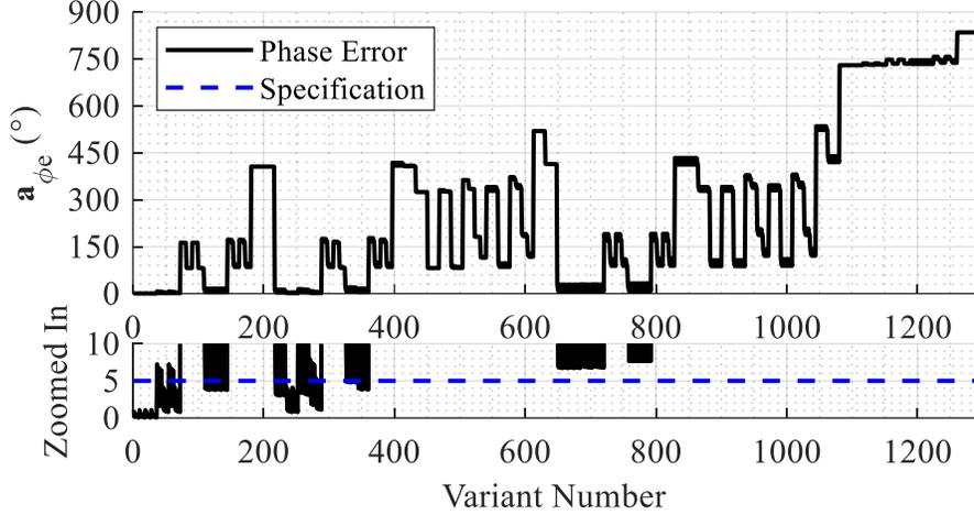
Figure 5.9 Demonstration of the non-linear relationship between RMS phase error and the variant number for the  $10 \times 6$  element PAA.
