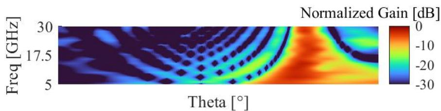
Figure 3.24 Normalized array pattern vs. scan angle and frequency for the TDU-A defined in Fig. 3.12 from model when including delay error steered to 50°.
