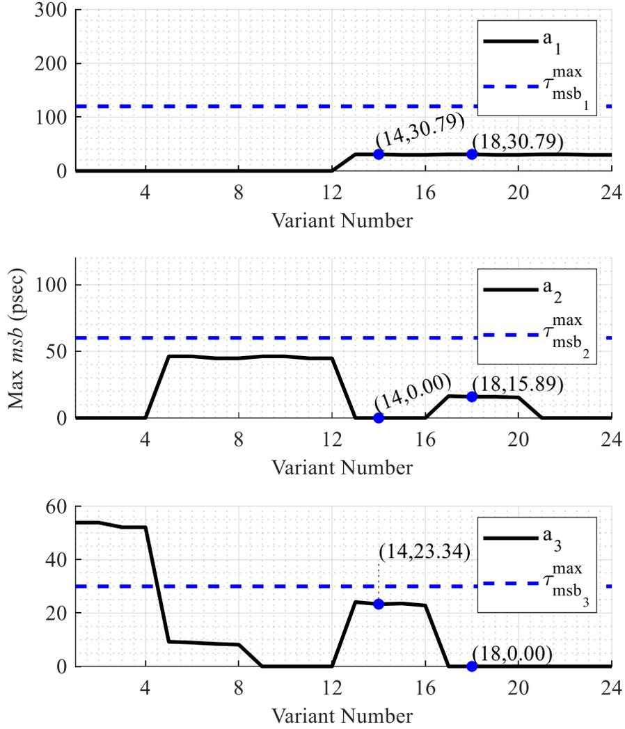
Figure 2.10 Demonstration of the non-linear relationship between the max *msb* for each level of division and the variant number for the 8 element PAA.
