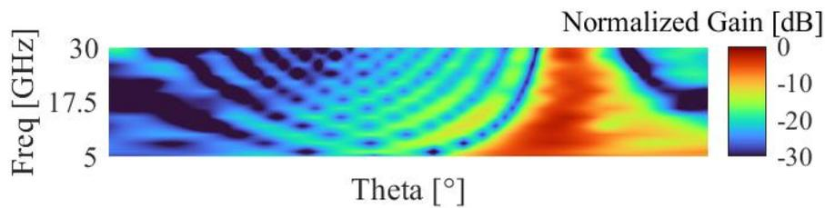
Figure 3.23 Normalized array pattern vs. scan angle and frequency for the TDU-A defined in Fig. 3.12 from model without including delay error steered to 50°.
