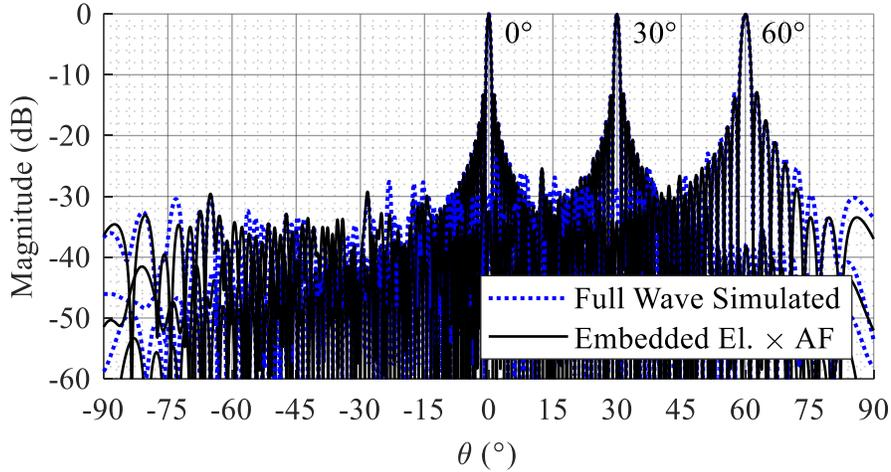
Figure 2.24 Normalized full wave simulated 128 element PAA pattern compared with [embedded element  $\times$  AF] pattern at  $f = 30$  GHz employing the optimum TDU architecture shown in Fig. 2.13.
