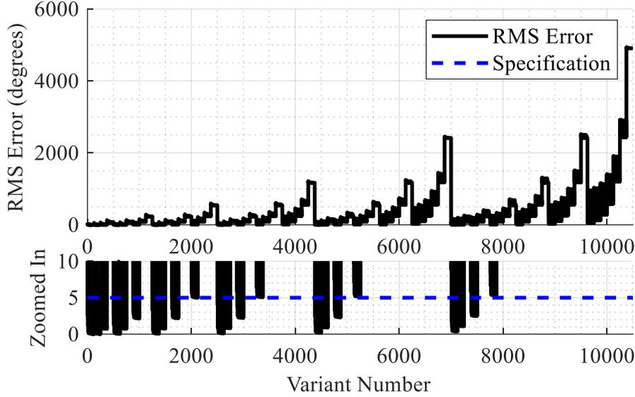
Figure 2.11 RMS phase error vs. variant number in the 128 element PAA.
