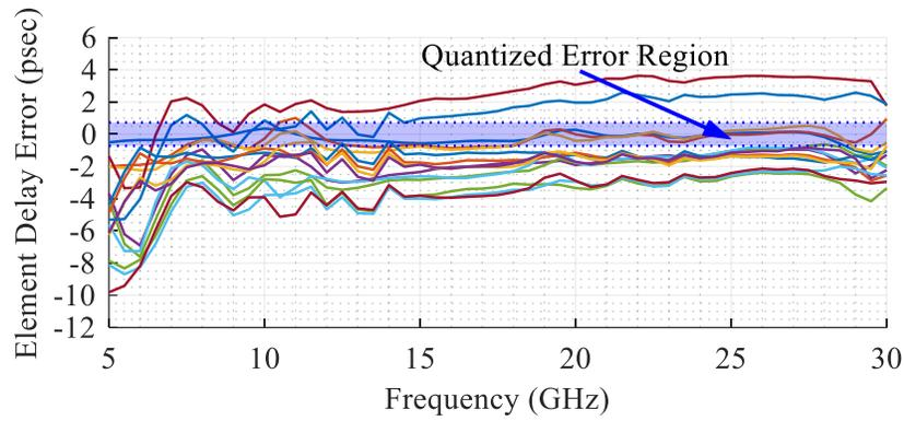
Figure 4.5 Distribution of delay error of the EM simulated TDU-A excitations for each element when compared to an ideal excitation before calibration.
