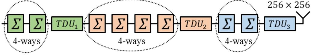
Figure 2.17 TDU architecture variant 7395 of the  $256 \times 256$  element PAA where  $TDU_1$  has 2 bits and  $\tau_{lsb} = 1306.4$  psec,  $TDU_2$  has 5 bits and  $\tau_{lsb} = 60.6$  psec, and  $TDU_3$  has 6 bits and  $\tau_{lsb} = 1.5$  psec.
