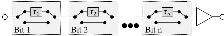
Figure 2.1 A TDU with  $n$  bits each with  $\tau_n$  of delay and an amplifier.
