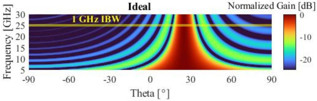
Figure 4.1 Array factor vs frequency of a 16 element array with ideal excitations.
