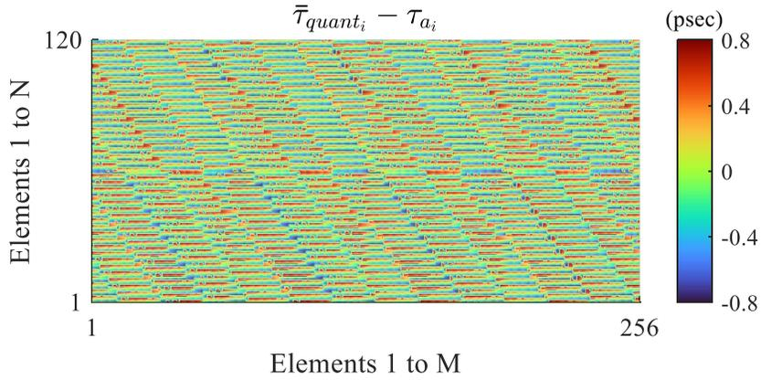
Figure A.9 Quantized delay error distribution for the TDU configurations of the architecture in Fig. 5.11 for a  $256 \times 120$  element PAA steered to  $\theta_{zx} = 60^\circ$  and  $\theta_{zy} = 30^\circ$ . Note that all element quantized error falls between  $\pm 0.8$  psec which satisfies the bounding  $\pm \tau_{lsb_2}/2$  criteria.
