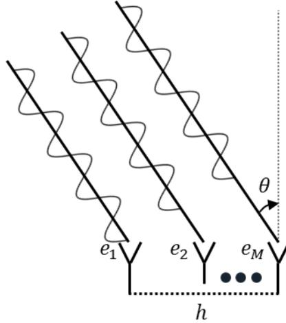
Figure 2.7 Illustration of maximum element distance for a linear array when a single TDU layer is placed directly under elements.
