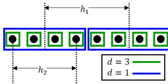
Figure 2.8 Illustration of maximum element distance for a linear array when two TDU layers are placed in the 8 element PAA architecture variant shown in Fig. 2.3.
