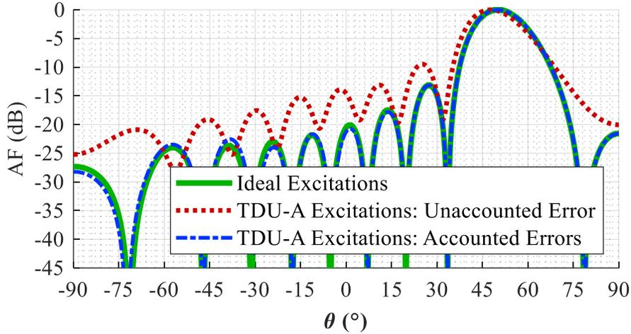
Figure 3.3 Effect of time delay errors from component non-idealities for the TDU-A shown in Fig. 3.2 at  $f_c = 17.5$  GHz in the array factor (AF) patterns with ideal excitations and excitations from the TDU-A when optimized with the time delay errors accounted or not.
