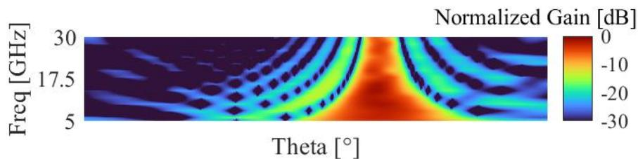
Figure 3.20 Normalized array pattern vs. scan angle and frequency for the TDU-A defined in Fig. 3.12 from model without including delay error steered to  $25^\circ$ .
