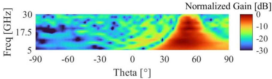
Figure 3.25 Normalized array pattern vs. scan angle and frequency for the TDU-A defined in Fig. 3.12 measured patterns from hardware steering to 50°.
