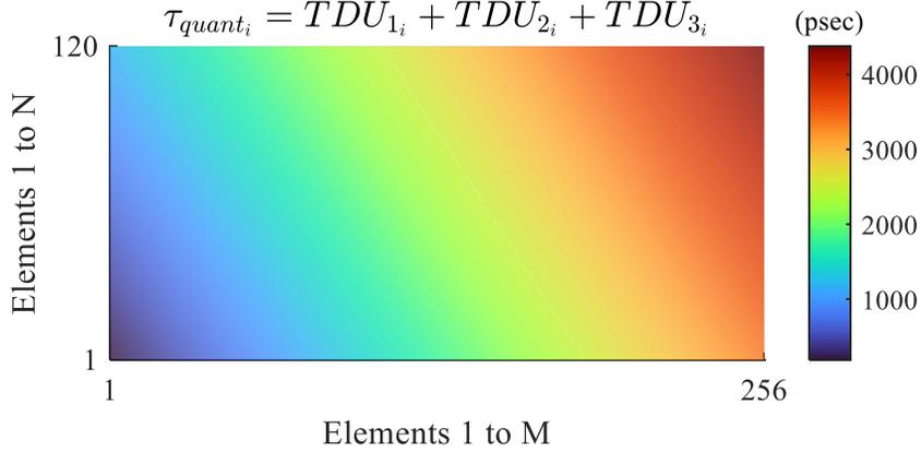
Figure A.7 Discretized total delay distribution for the TDU configuration of the architecture in Fig. 5.11 for a  $256 \times 120$  element PAA steered to  $\theta_{zx} = 60^\circ$  and  $\theta_{zy} = 30^\circ$ .
