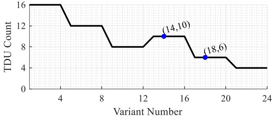
Figure 2.5 TDU count vs variant number of the 8 element PAA. Data points correspond to variants shown in Figs. 2.3 and 2.4.
