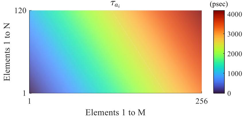
Figure A.1 Ideal delay settings for each element of a  $256 \times 120$  element PAA steered to  $\theta_{zx} = 60^\circ$  and  $\theta_{zy} = 30^\circ$ .
