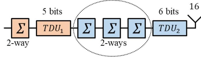
Figure 3.12 Optimized TDU architecture of the 16 element linear PAA where  $TDU_1$  has 5 bits and  $\tau_{lsb} = 4.4$  psec and  $TDU_2$  has 6 bits and  $\tau_{lsb} = 1.45$  psec.
