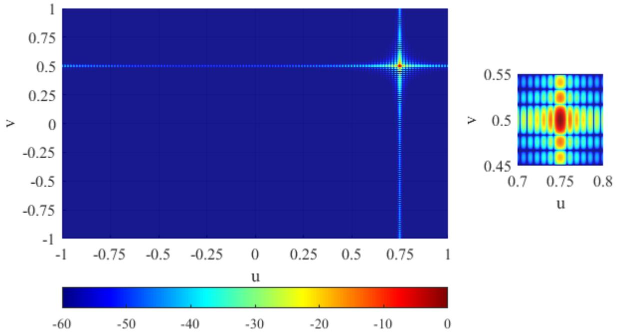
Figure 5.13 AF of  $256 \times 120$  PAA scanned to  $\theta_{zx_{max}} = 60^\circ$  and  $\theta_{zy_{max}} = 30^\circ$  with excitations that are ideal.
