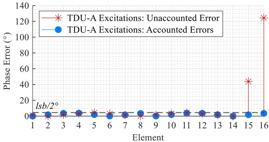
Figure 3.4 Effect of time delay errors from component non-idealities for the TDU-A shown in Fig. 3.2 at  $f_c = 17.5$  GHz in the absolute value of the phase error across antenna elements.
