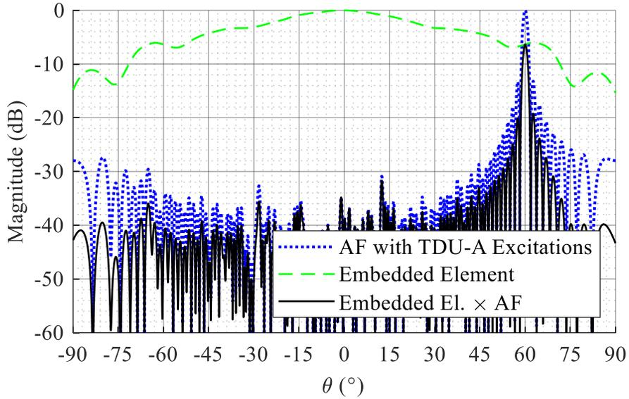
Figure 2.22 Normalized patterns for the 128 element Vivaldi antenna array at 30 GHz with a 60° scan.
