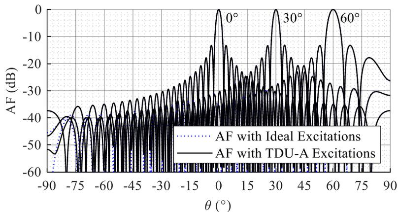
Figure 2.15 Normalized array factor of 128 element linear PAA at  $f = 10$  GHz when it employs the optimum TDU architecture (TDU-A) excitations shown in Fig. 2.13 and ideal excitations.
