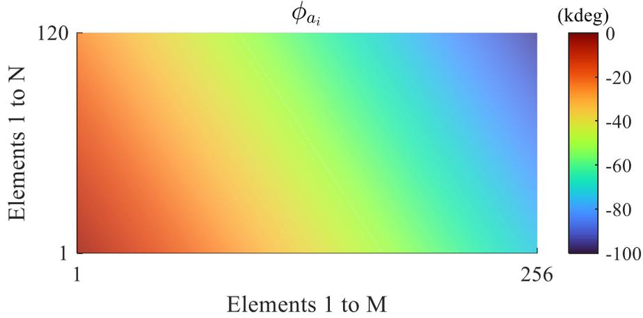
Figure A.10 Phase distribution for the TDU configurations of the architecture in Fig. 5.11 for a  $256 \times 120$  element PAA steered to  $\theta_{zx} = 60^\circ$  and  $\theta_{zy} = 30^\circ$  at  $f = 30$  GHz.
