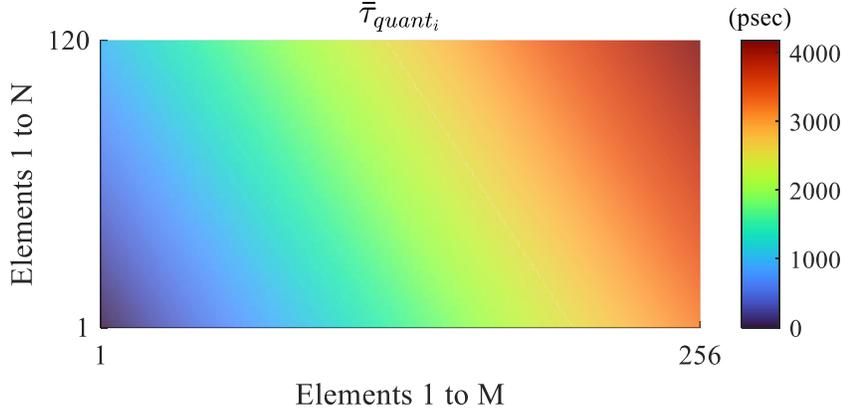
Figure A.8 Normalized discretized total delay distribution for the TDU configuration of the architecture in Fig. 5.11 for a  $256 \times 120$  element PAA steered to  $\theta_{zx} = 60^\circ$  and  $\theta_{zy} = 30^\circ$ .
