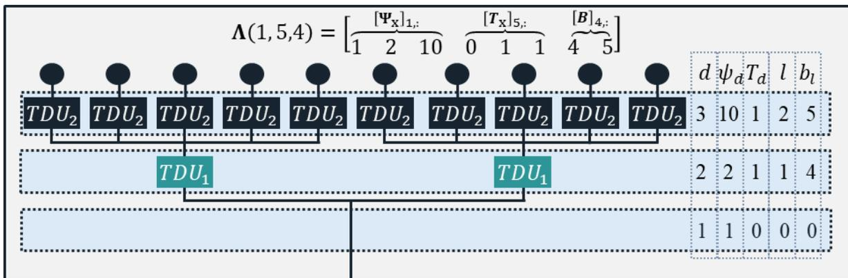
Figure 5.6 Architecture variant examples for a  $D_x = 3$  division level 10 element PAA with a 2-way divider followed by a 5-way divider with a 4 bit TDU layer in  $d = 2$  and 5 bit TDU layer in  $d = 3$  with no TDU in  $d = 1$ .
