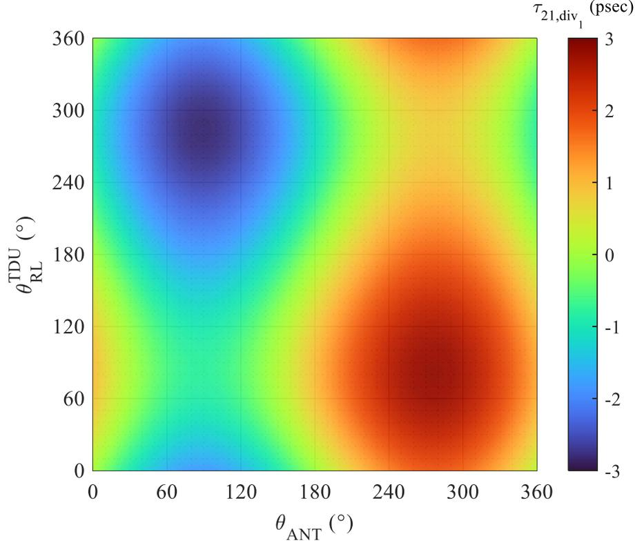
Figure 3.7 Time delay variation at 5 GHz when the divider is terminated with  $\Gamma_{L2} = \Gamma_{L3} = 0.178 e^{-j\theta_{RL}^{TDU}}$  and  $\angle\Gamma_{L2}$  and  $\angle\Gamma_{L3}$  are swept independently.
