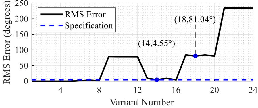
Figure 2.9 Demonstration of the non-linear relationship between RMS phase error and the variant number for the 8 element PAA.
