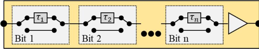
Figure 3.1 A TDU block diagram with  $n$  bits, each with  $\tau_n$  of delay capability.
