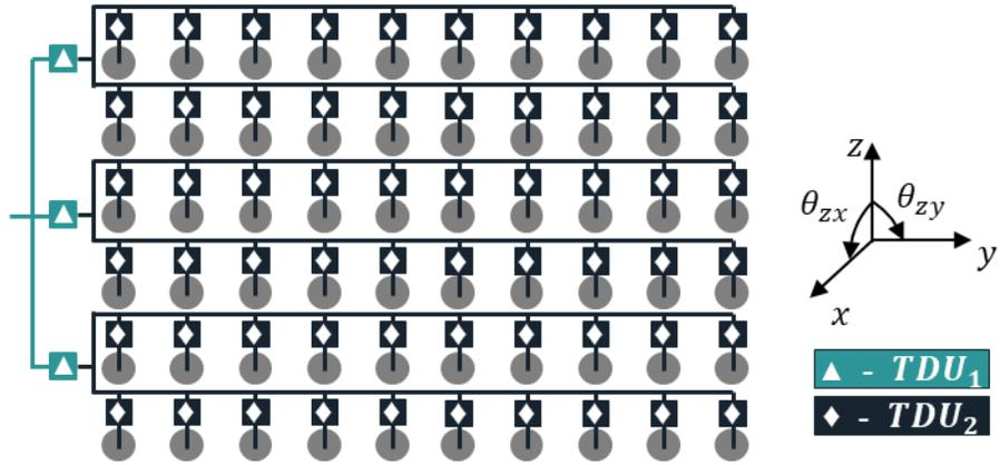
Figure 5.1 Demonstrating the TDU-A for a  $10 \times 6$  PAA graphically for configuration vector  $\Lambda(2,2,4,5,7)$  or  $[\mathbf{Y}]_{v=1177, \dots}$
