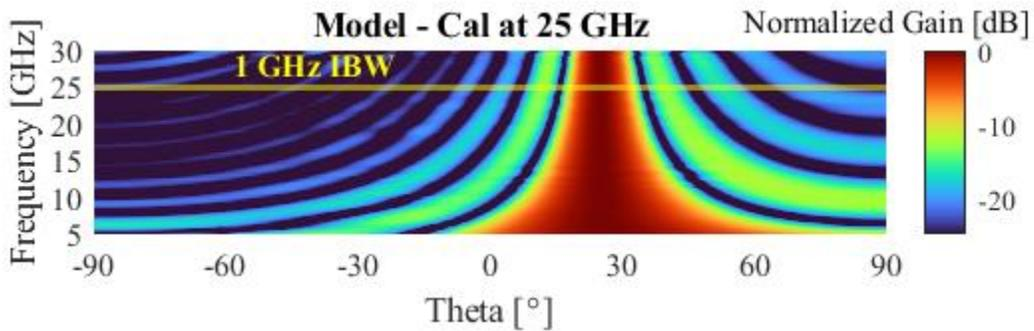
Figure 4.3 Array factor vs frequency of a 16 element array with calibrated EM TDU-A simulated excitations at 25 GHz with a 1 GHz IBW.
