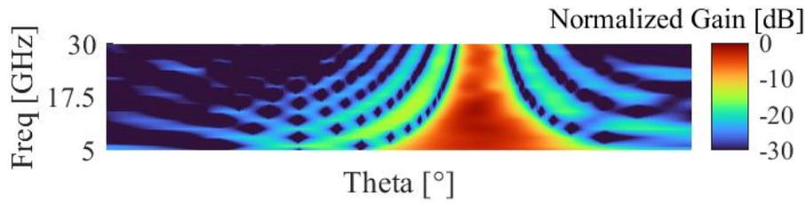
Figure 3.21 Normalized array pattern vs. scan angle and frequency for the TDU-A defined in Fig. 3.12 from model when including delay error steered to 25°.
