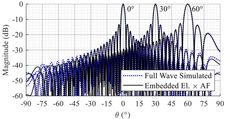
Figure 2.23 Normalized full wave simulated 128 element PAA pattern compared with [embedded element × AF] pattern at  $f = 10$  GHz employing the optimum TDU architecture shown in Fig. 2.13.
