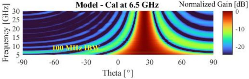
Figure 4.4 Array factor vs frequency of a 16 element array with calibrated EM TDU-A simulated excitations at 6.5 GHz with a 100 MHz IBW.
