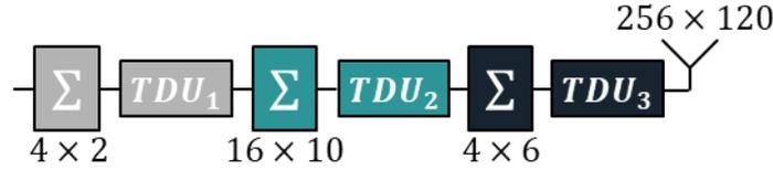
Figure 5.11 TDU-A variant 8318050 of the  $256 \times 120$  element PAA where  $TDU_1$  has 3 bits and  $\tau_{lsb} = 431.7$  psec,  $TDU_2$  has 6 bits and  $\tau_{lsb} = 22.7$  psec, and  $TDU_3$  has 6 bits and  $\tau_{lsb} = 1.6$  psec.
