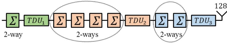
Figure 2.13 Optimum TDU architecture for the 128 element PAA where  $TDU_1$  has 2 bits and  $\tau_{lsb} = 307.9$  psec,  $TDU_2$  has 4 bits and  $\tau_{lsb} = 68.0$  psec, and  $TDU_3$  has 6 bits and  $\tau_{lsb} = 1.2$  psec.
