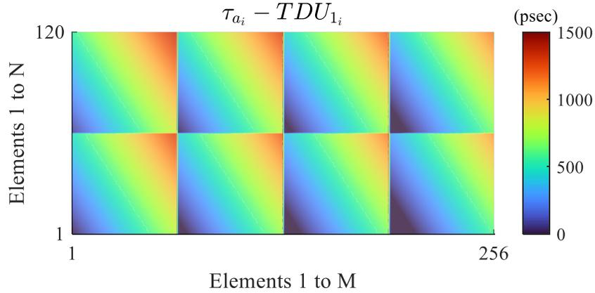
Figure A.3 Delay delta to be made up for by the remaining TDU layers after layer 1 in the architecture in Fig. 5.11 for a  $256 \times 120$  element PAA steered to  $\theta_{zx} = 60^\circ$  and  $\theta_{zy} = 30^\circ$ .
