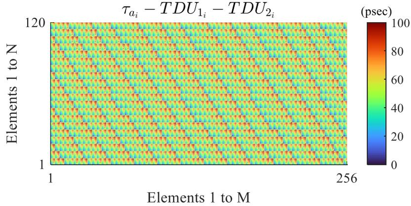
Figure A.5 Delay delta to be made up for by the remaining TDU layers after layer 2 in the architecture in Fig. 5.11 for a  $256 \times 120$  element PAA steered to  $\theta_{zx} = 60^\circ$  and  $\theta_{zy} = 30^\circ$ .
