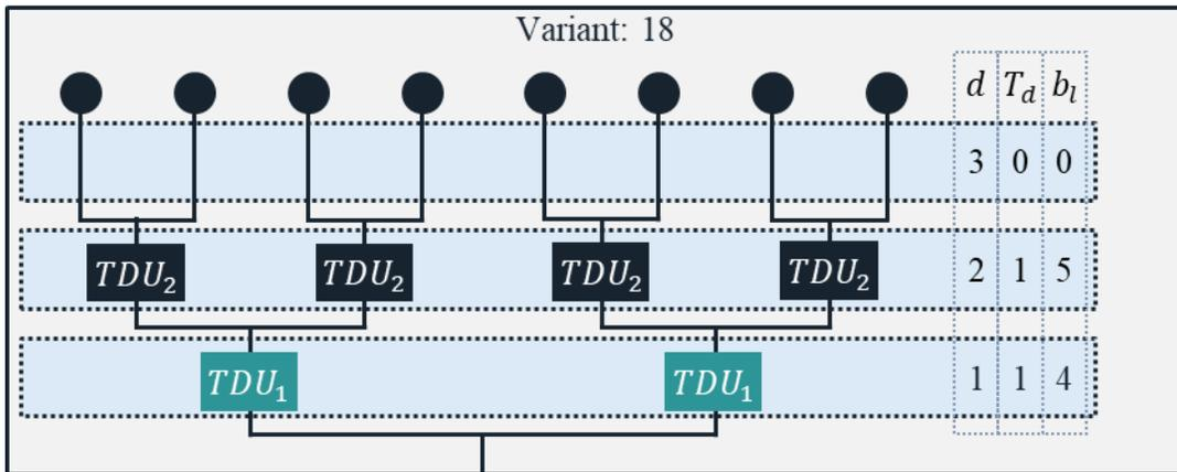
Figure 2.4 Architecture variant example for a  $D = 3$  division level 8 element PAA with a 5 bit TDU layer in  $d = 2$  and a 4 bit TDU layer in  $d = 1$  with no TDUs in  $d = 3$ .
