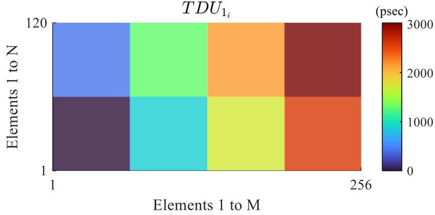
Figure A.2 TDU settings for layer 1 of the architecture in Fig. 5.11 for a  $256 \times 120$  element PAA steered to  $\theta_{zx} = 60^\circ$  and  $\theta_{zy} = 30^\circ$ .
