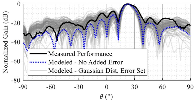
Figure 3.27 Comparison of 18 GHz measurement (bold plots) vs 100 iterations of modeled performance (light gray plots) within the family of expected delay errors in the RF-fanout steered to 25°.
