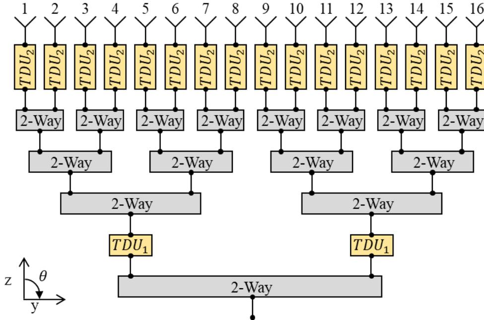
Figure 3.2 An example TDU architecture for a 16 element PAA (which is also the optimal for the PAA and its requirements considered in this chapter).
