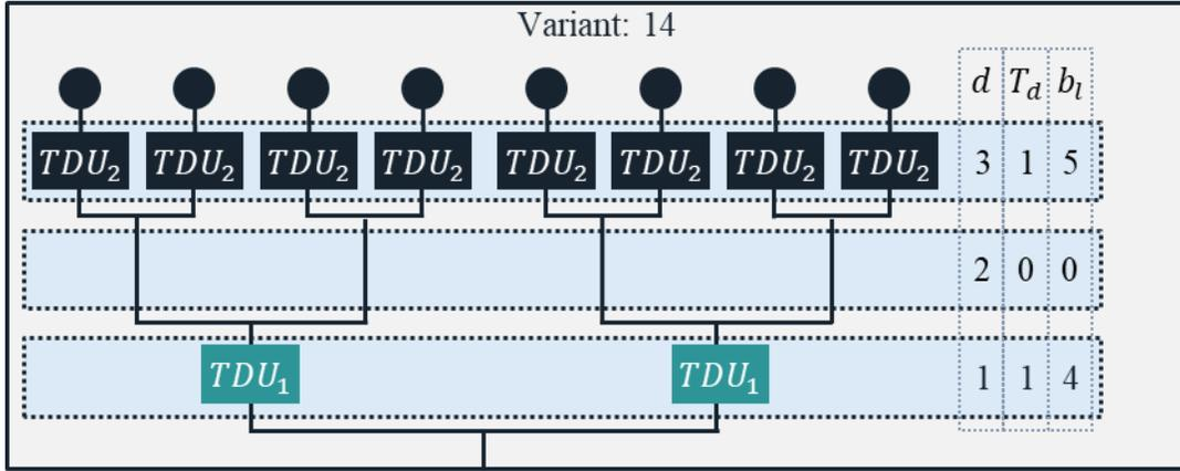
Figure 2.3 Architecture variant example for a  $D = 3$  division level 8 element PAA with a 5 bit TDU layer in  $d = 3$  and a 4 bit TDU layer in  $d = 1$  with no TDU in  $d = 2$ .
