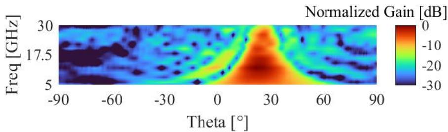
Figure 3.22 Normalized array pattern vs. scan angle and frequency for the TDU-A defined in Fig. 3.12 measured patterns from hardware steering to 25°.
