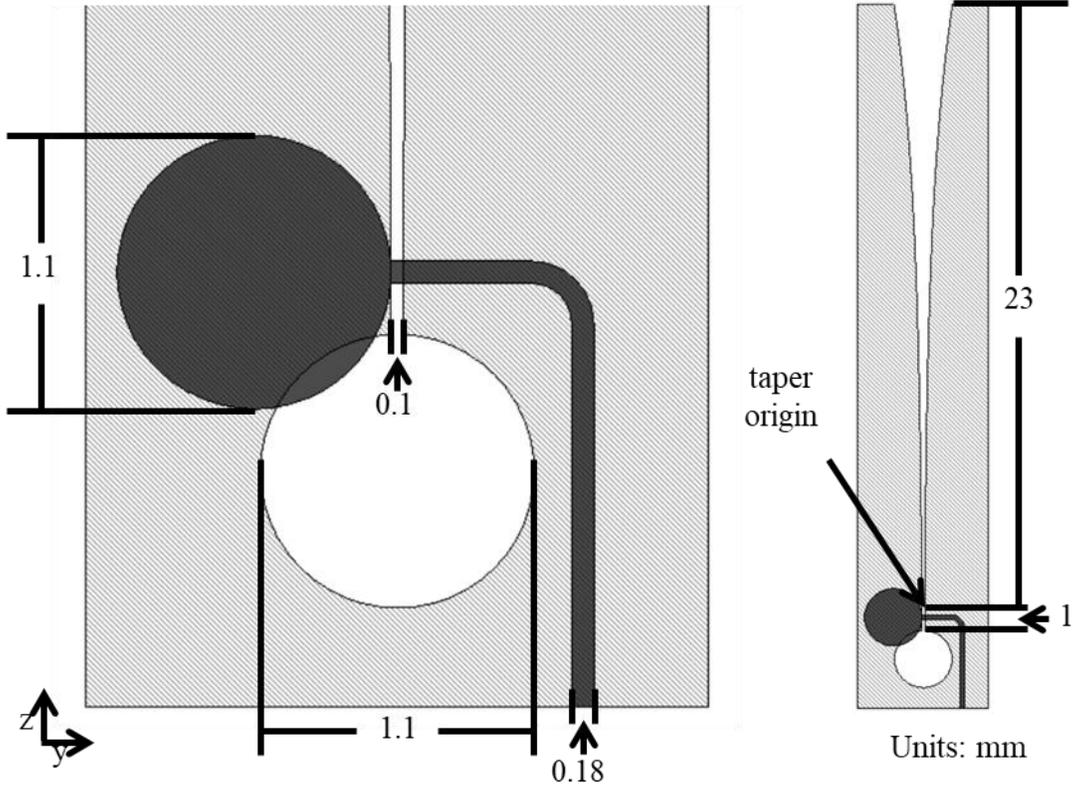
Figure 2.20 Antenna element geometry (dimensions are in mm).
