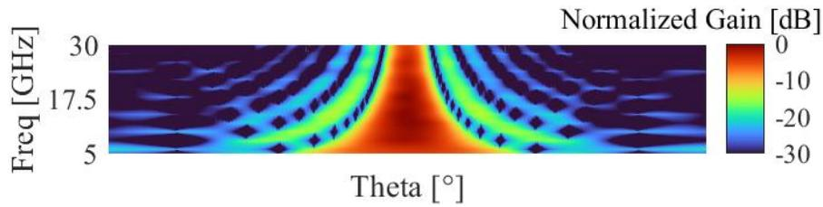
Figure 3.17 Normalized array pattern vs. scan angle and frequency for the TDU-A defined in Fig. 3.12 from model without including delay error steered to  $0^\circ$ .
