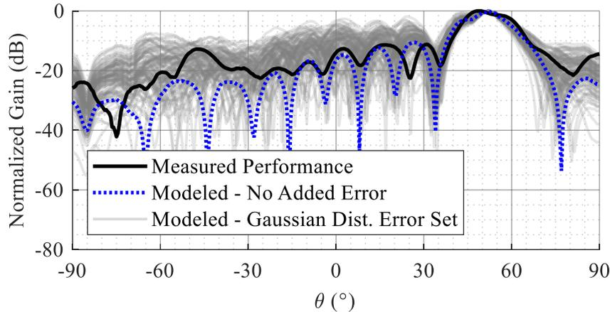
Figure 3.28 Comparison of 18 GHz measurement (bold plots) vs 100 iterations of modeled performance (light gray plots) within the family of expected delay errors in the RF-fanout steered to 50°.
