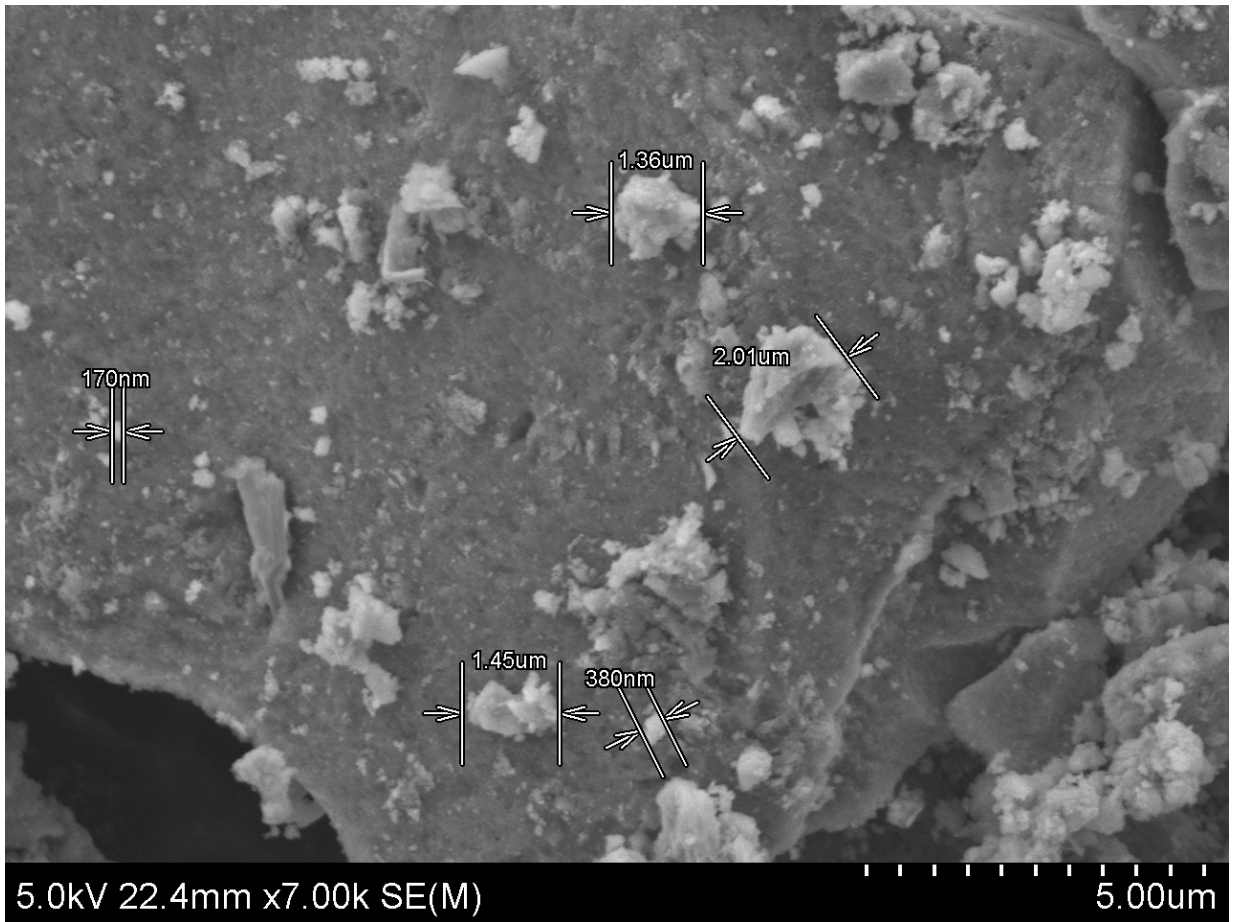
Figure 16: 10% MoS 2 -90% TiO 2 SEM readout #2.
