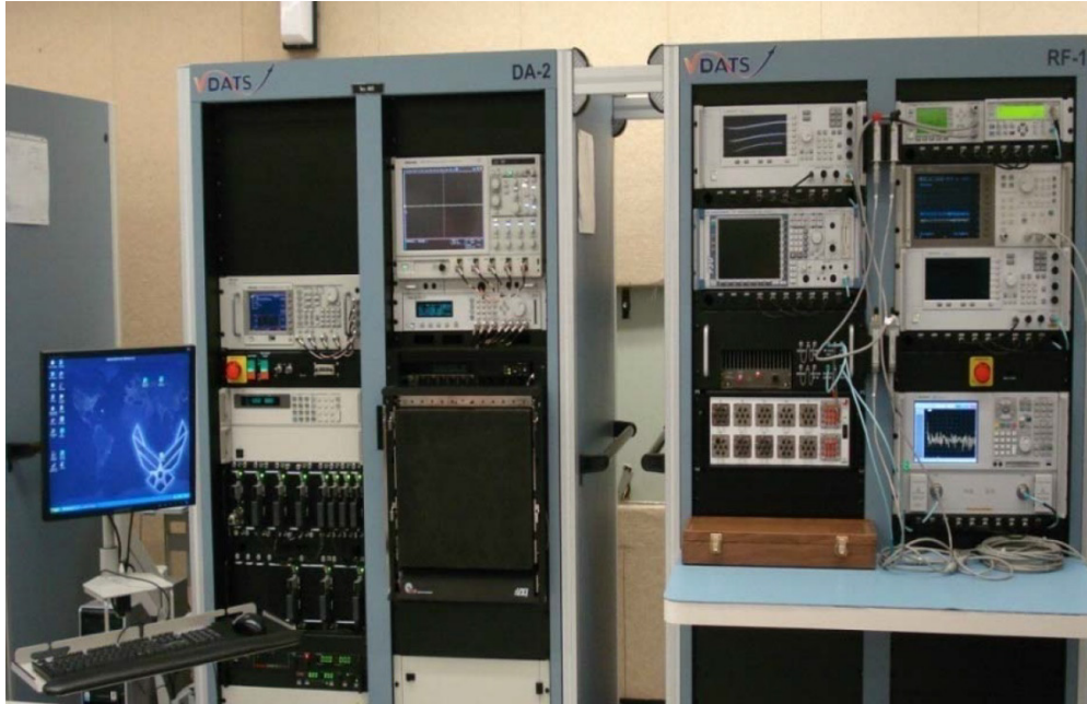
Figure 1.3 VDATS Core Variants: Digital-Analog (DA, Left) and Radio Frequency (RF, Right)
