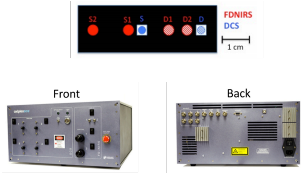
Figure 4.1: A hybrid multi-distance DOS and DCS probe and corresponding system. Figure adapted with permission from [19].
