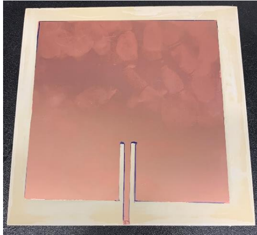
Figure 5-13 Micrograph of a dielectric patch antenna designed and milled using Rogers RO3010 laminate as the substrate.
