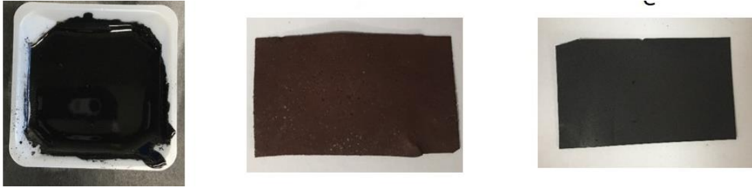
Figure 2-3 NiCuZn ferrite slurry with unsintered and sintered sheet.
