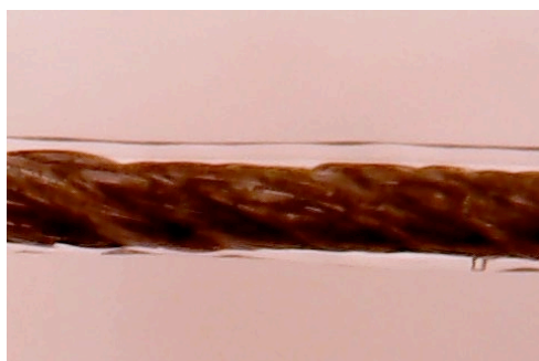
Figure S3: Jameco thread coated with a layer of gel electrolyte before making the twisted-fiber capacitor.
