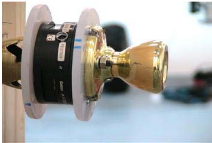
Figure 4.3. ATI TM Gamma transducer connected to the door knob.
