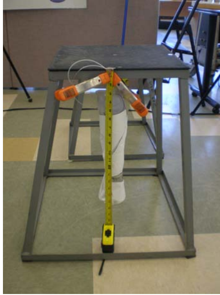
Figure 6.2. Suspension test on a typical TRMP to determine inertial properties.
