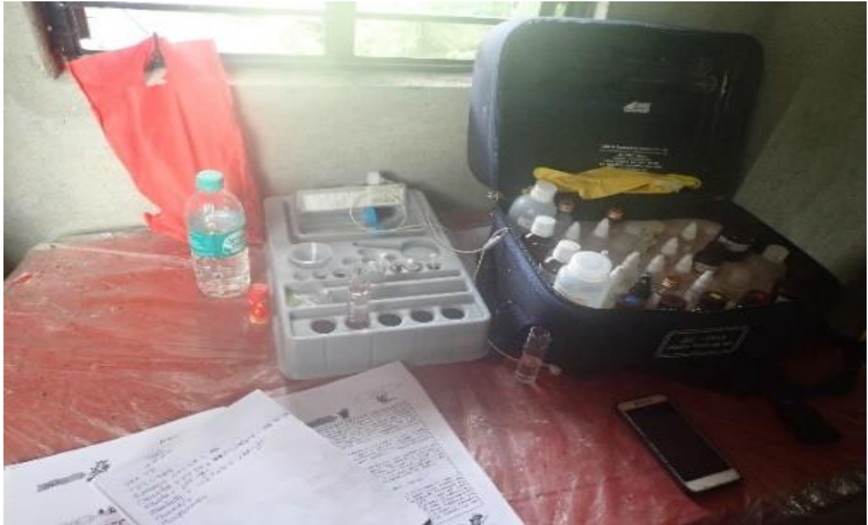
Figure 3. Water Testing Kit for the Water Treatment Plant
