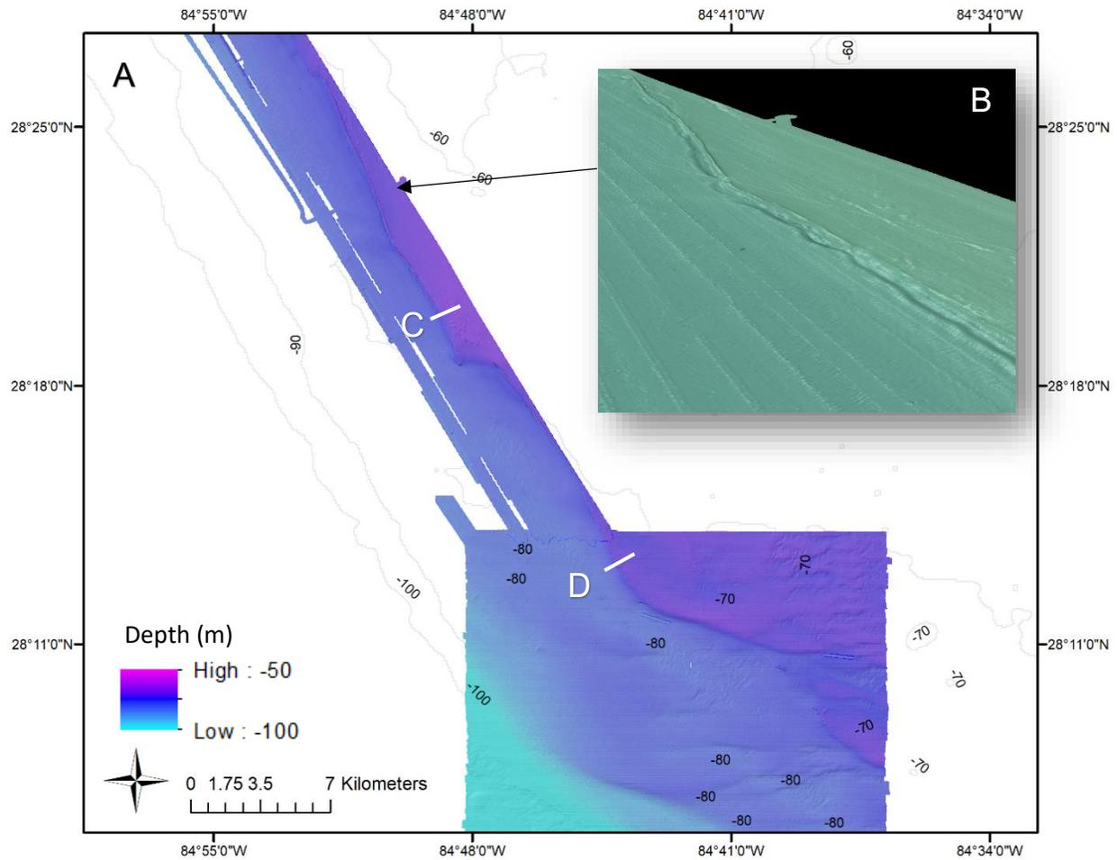
**Figure 12:** (A) Shoreline 11 – The Edges and Steamboat Lumps MPA’s. (B) 3D close-up of trough running parallel to ridges on seaward side. (C,D) Cross-sections (10x exaggeration) through shoreline 11 showing a prominent ridge and seaward depression in the north which becomes more rounded and smooth to the south.
