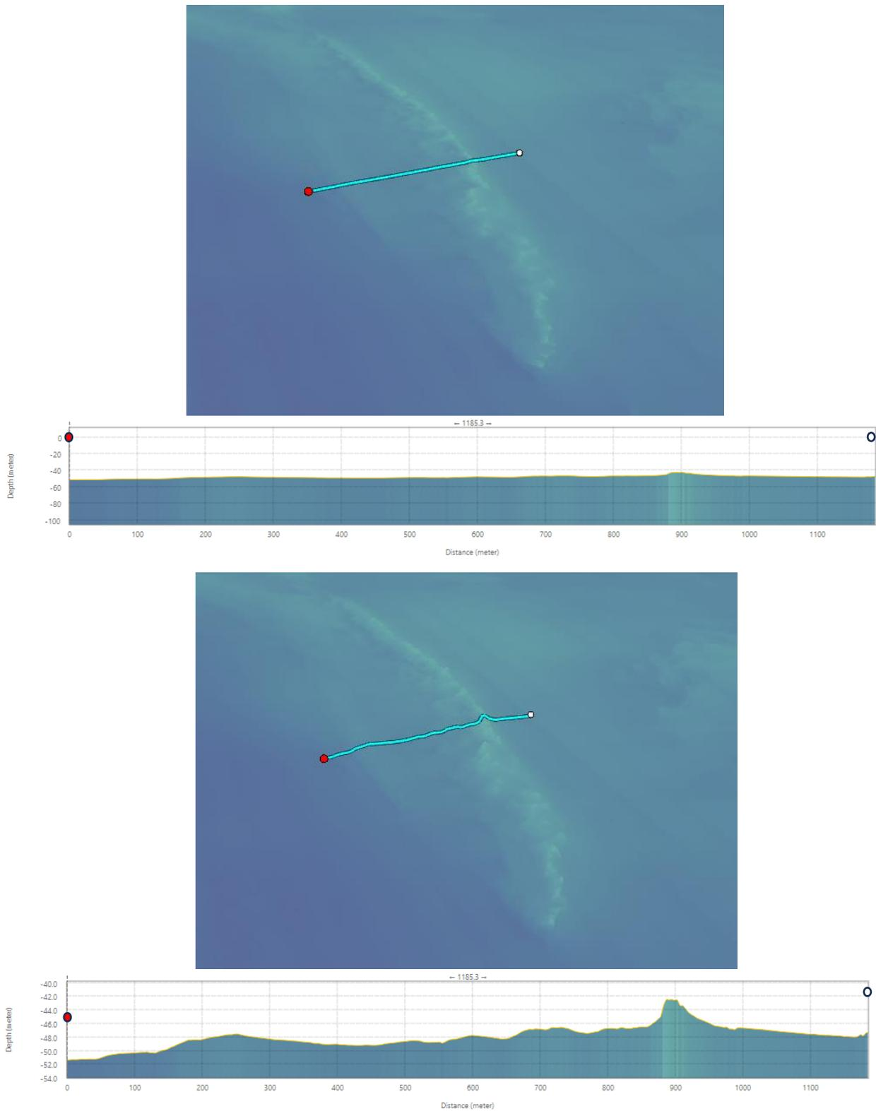
**Figure 6:** An example of the same paleoshoreline feature (from the SW Florida Middle Grounds) with no vertical exaggeration (A) and using 10x vertical exaggeration (B) to illustrate the usefulness of this technique in identifying subfeatures that would otherwise be indiscernible due to the subtlety of their seafloor expression.
