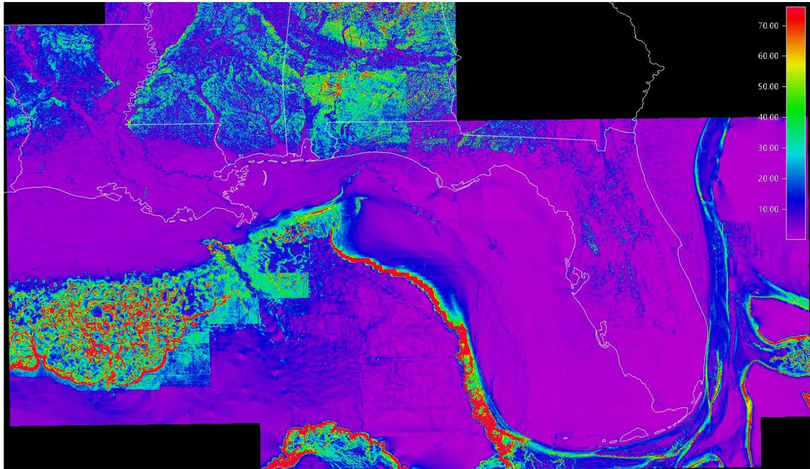
**Figure 3:** Slope map of the north and eastern Gulf of Mexico highlighting the extent and gradient of the West Florida Shelf. Color legend is degrees of slope. Note location of De Soto Canyon which marks the boundary between siliciclastic sediments from the Mississippi River to the west, and carbonate sediments to the east.
