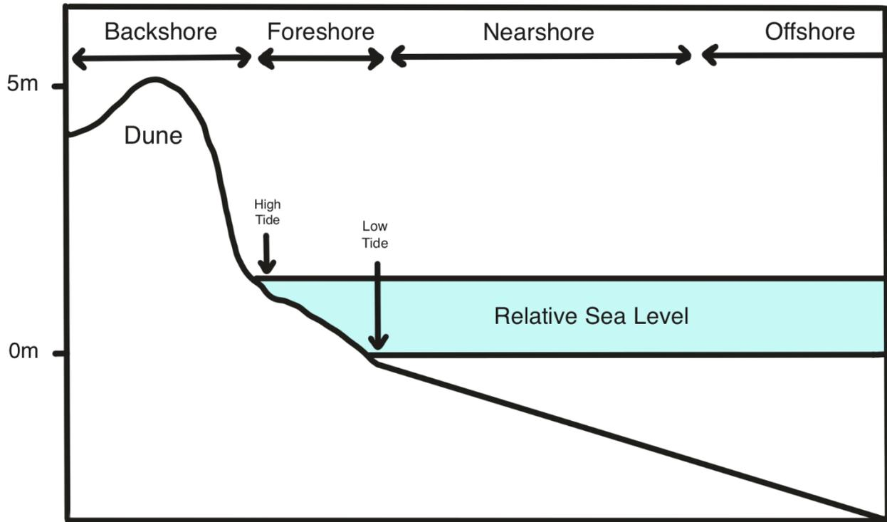
**Figure 7:** Beach profile highlighting foreshore and dune crest from which a window for deriving relative sea level values was based on (derived from Bird, 2000).
