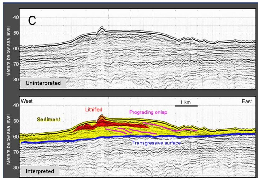
**Figure 14:** (A) Shoreline 13 – The Elbow. (B) Seismic profile track line over the SW Florida Middle Grounds and The Elbow from July-August 2018. (C) Interpretation of subbottom profile of The Elbow indicates the feature is a coastal spit structure containing probable beachrock and non-marine beach deposits (Dr. Stanley Locker, pers. comm.).
