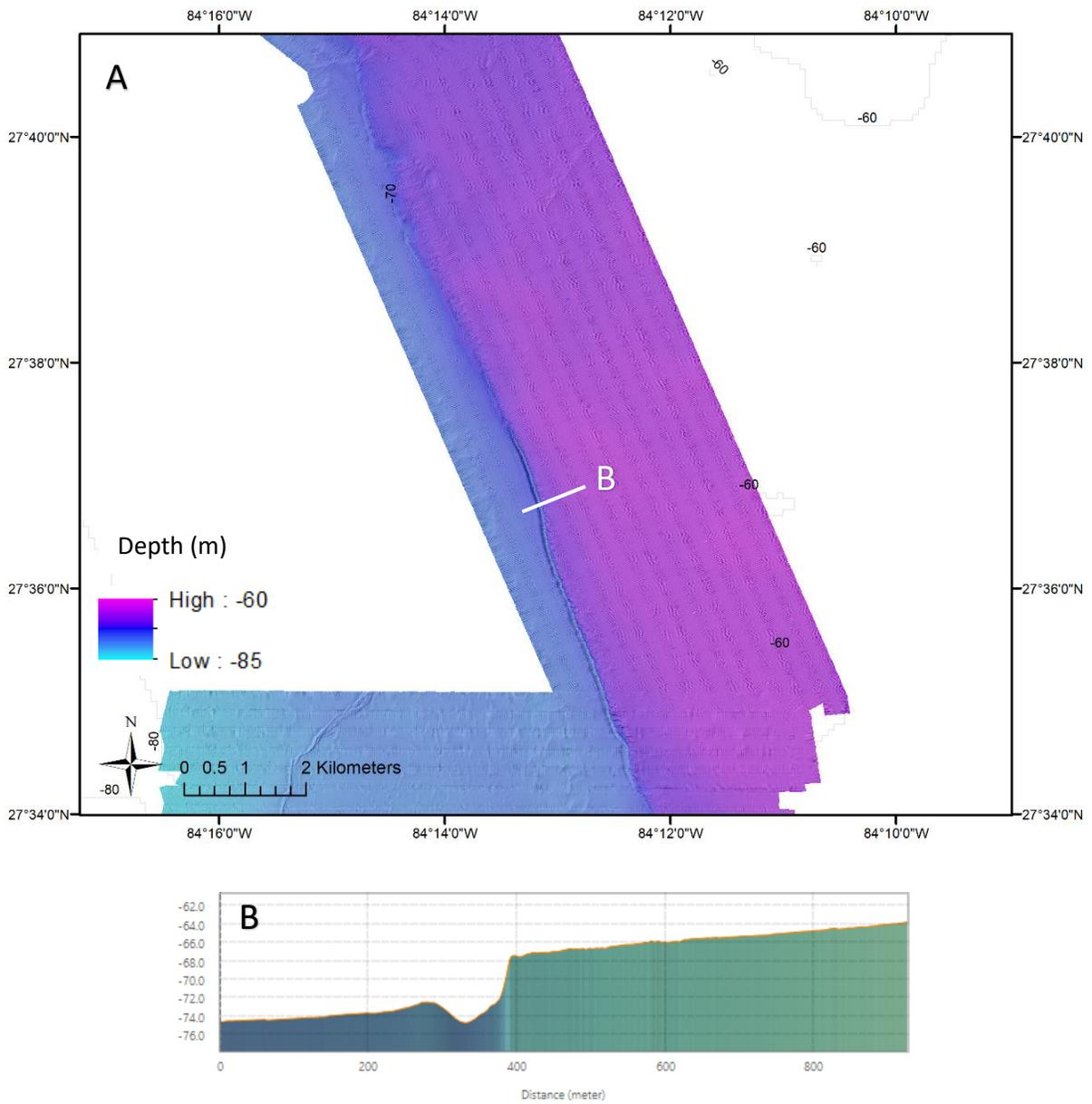
**Figure 16:** (A) Shoreline 16 – Radius-Ulna. (B) Cross-section showing the terrace that is speculated could be a former mangrove platform.
