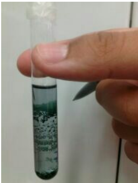
Figure 22: Photo of crystal formation from one test tube. stp crystals are the particles at the bottom of the test tube, though the largest crystals were attached on the side of the test tube. Courtesy of Joy D'Andrea.
