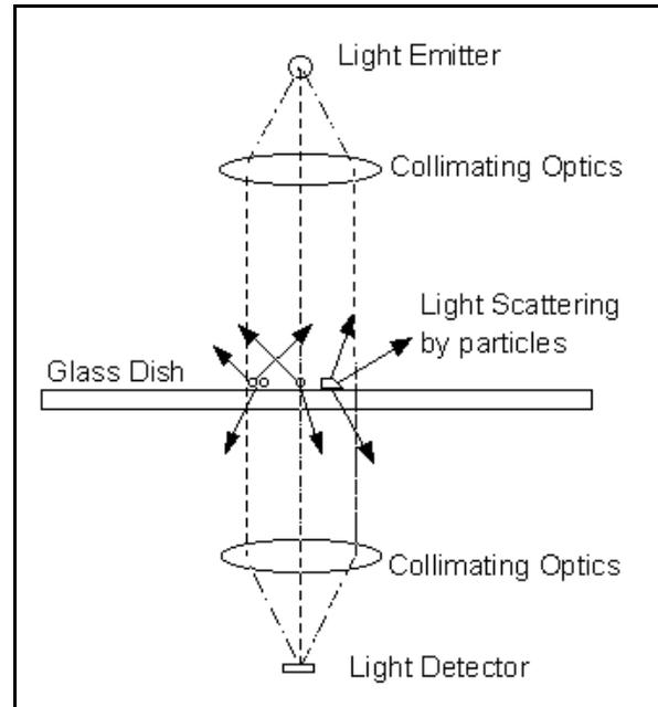
Figure 3. Optical system of the dust film measuring instrument.
