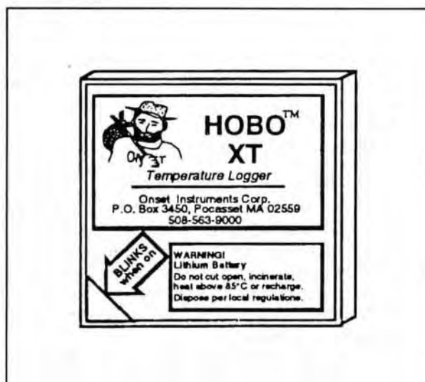
Figure 1. Actual size of the Hobo data temperature logger manufactured by Onset Instrument Corporation.
