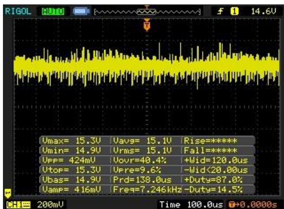
Figure 2.7: Output voltage waveform with no load conditions for XL6009
