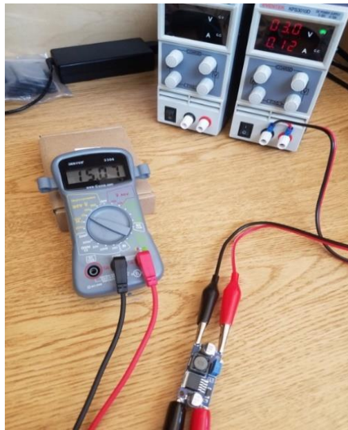
Figure 2.2: In-lab experimental setup for the off-the-shelf XL6009 DC-DC converter module under no load conditions
