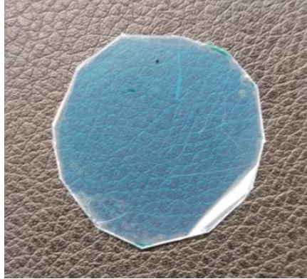
Figure 10: ITO sample used for sheet resistance measurement.
