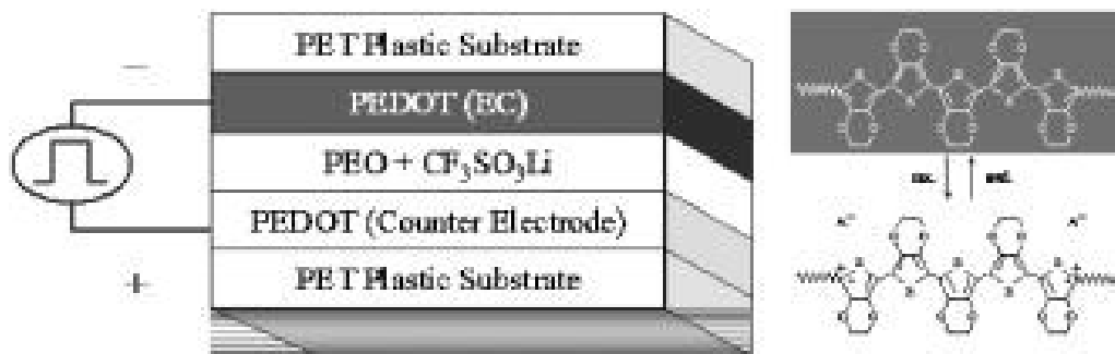
Figure 2-8 Multi-Layer Configuration of an Electrochromic Device [31]. By Ricardo Vergaz et al. © (2006) Society of Photo-Optical Instrumentation Engineers (SPIE).
