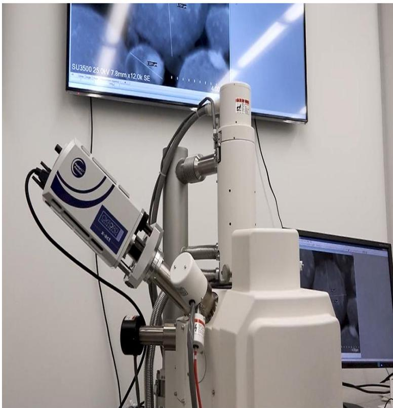
Figure 24: Scanning Electron Microscope (Hitachi SU3500) at Florida Polytechnic University.
