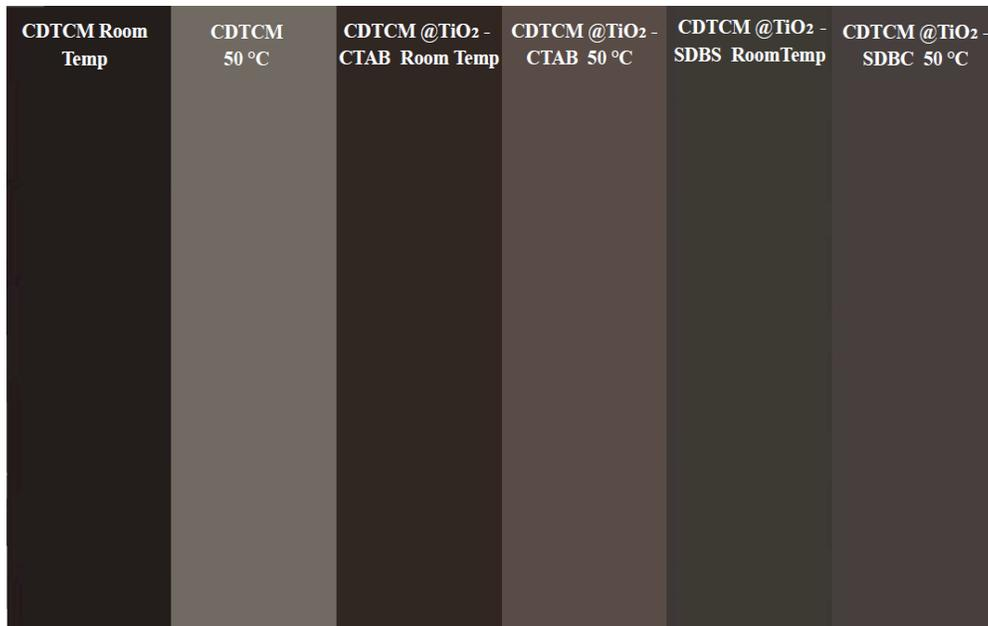
Figure 57: CIE LAB Color Simulation of the Samples at Room Temp & at 50 °C.
