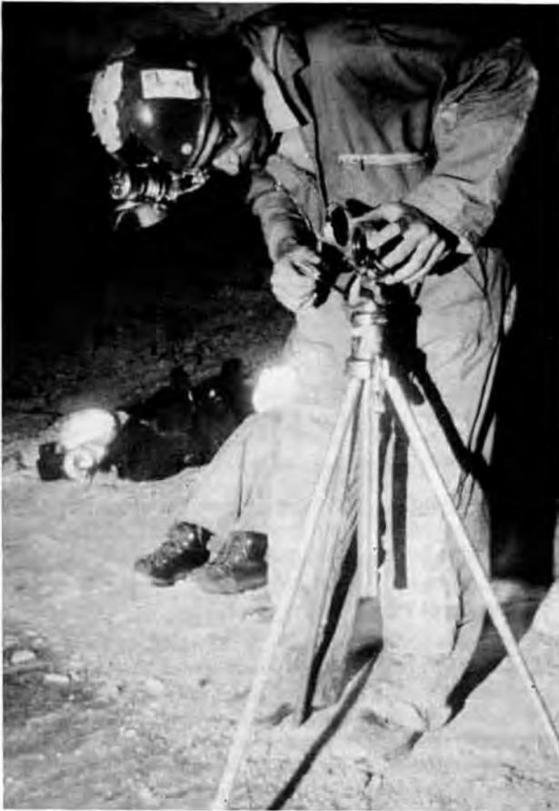
Figure 3. A Brunton compass is used to determine the vertical angle and azimuth of the camera face.
