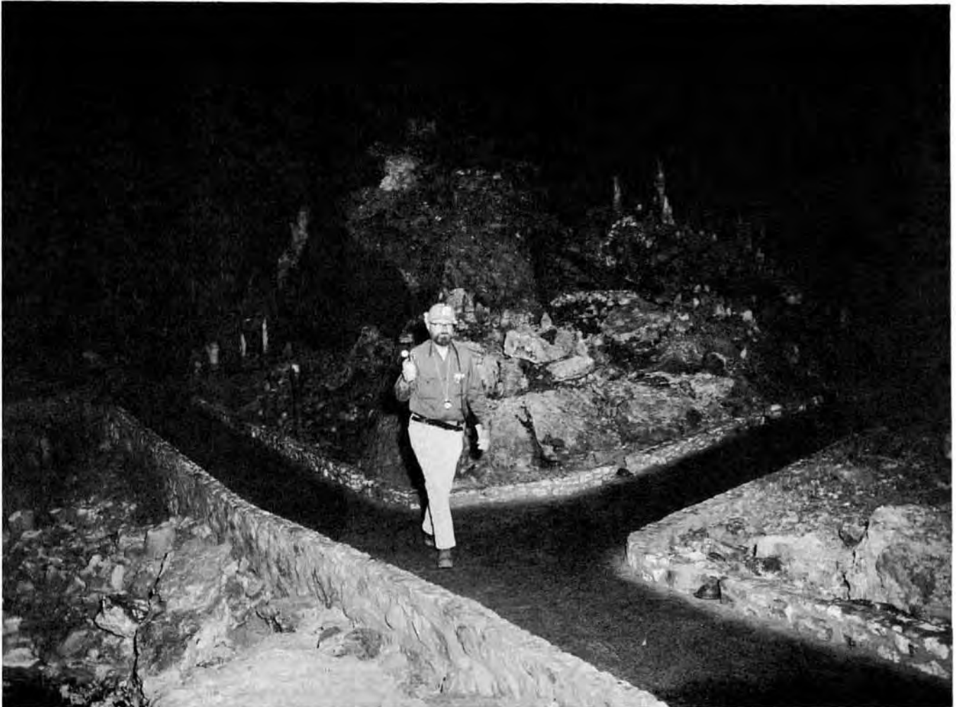
The author is shown here using the typical air pump and filter unit to collect a timed sample of cave air for airborne radiation determination. Photo by Charlie and Jo Larson.
