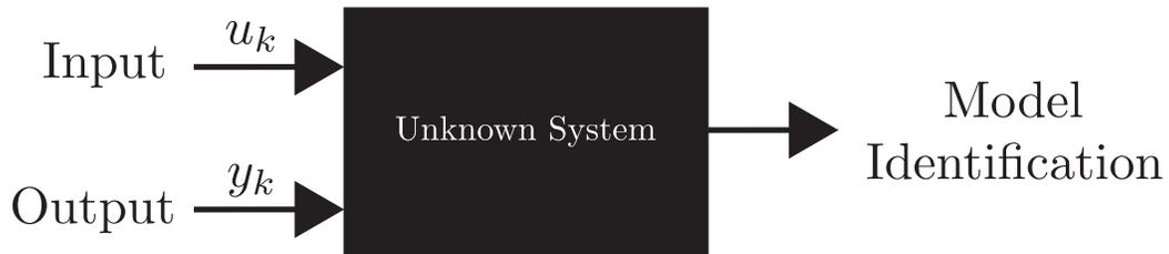
Figure 1.3: Black-box modeling scheme. It takes only the system input and output measurement to identify the system characteristics.
