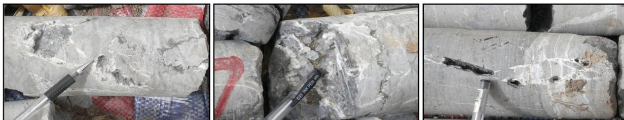
**Figure 5.** Cemented fractures in Fengfeng Formation.
