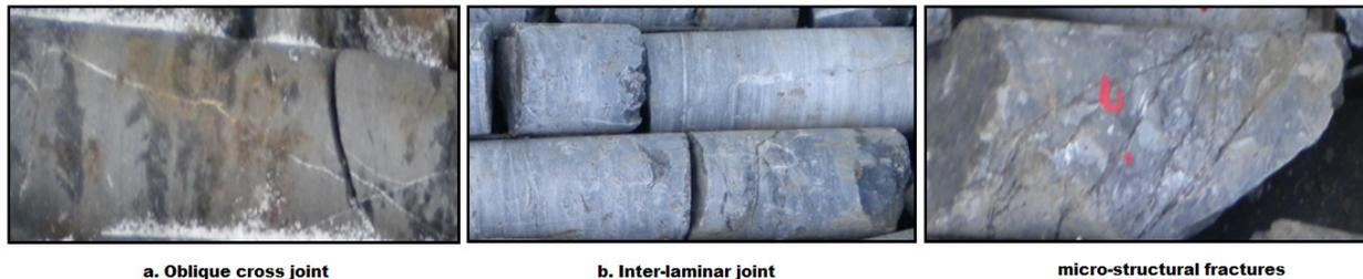
**Figure 4.** Three different types of fractures in Fengfeng Formation.
