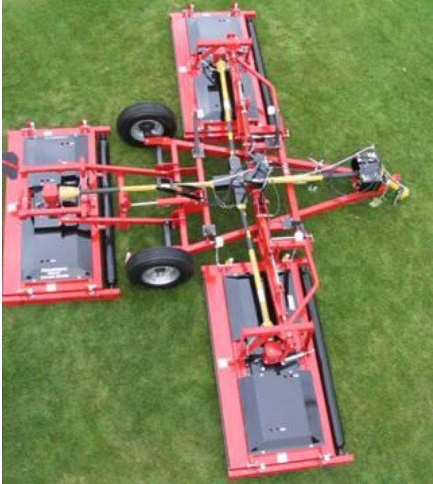
h. Figure 8: Tow-behind mower (does not move on its own, needs to be pulled)
