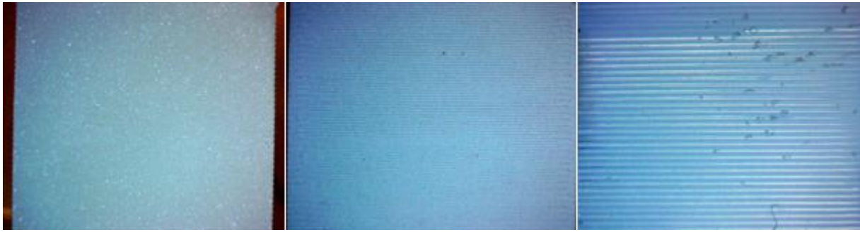
Figure 2.3 – CB028, Novacentrix FG57B, and Novacentrix FG77 dispensed onto Kapton tape in 10 mm squares.
