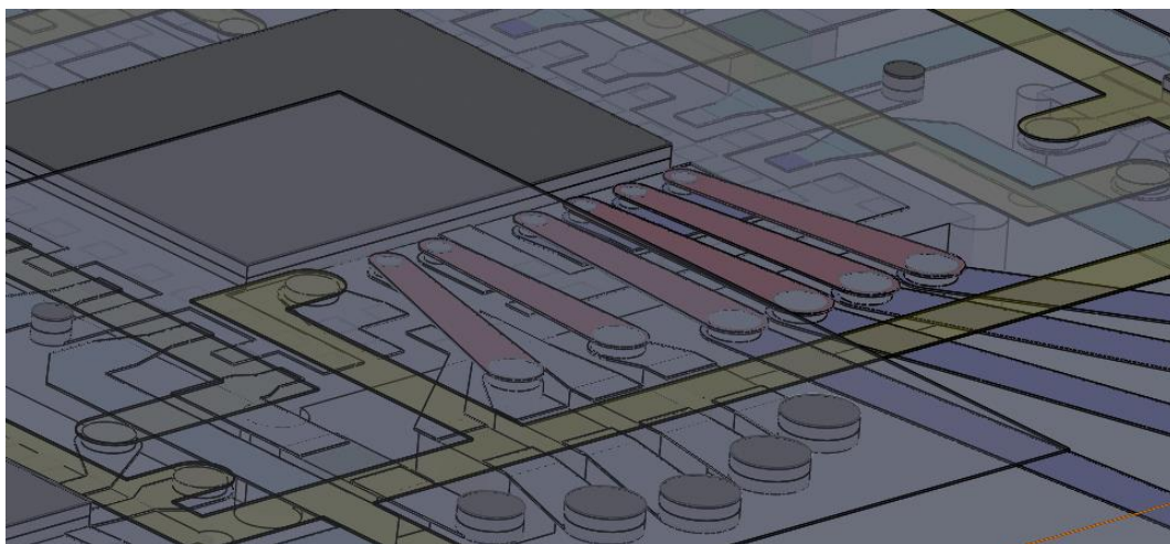
Figure 4.4 – On-chip via and temporary layer transition for 4-wire SPI. Critical fabrication point where issues were expected to be encountered.
