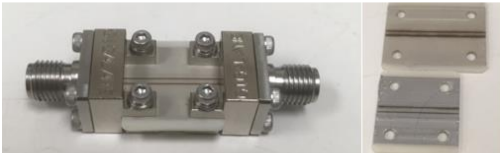
Figure 2.17 – CPW substrate with improved connectors (Left) and 10 mm CB028 and 5 mm FG77 substrates (Right).
