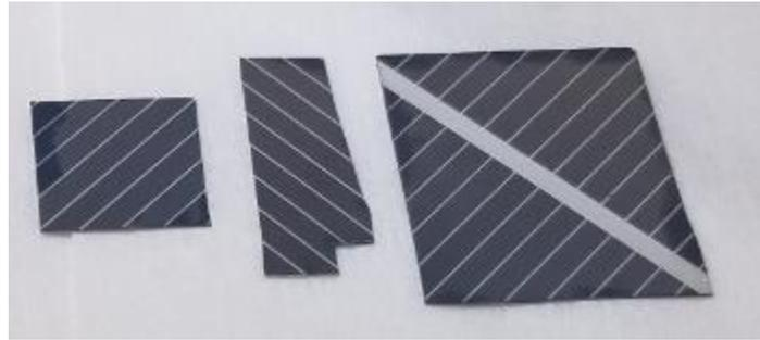
Figure 15: Solar cell after DRIE etch
