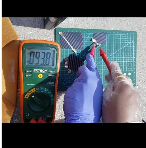
Figure 26: Solar cell scribed into 3.5 X 2.5 cm, and DRIE etched Coated with CoO ATO
