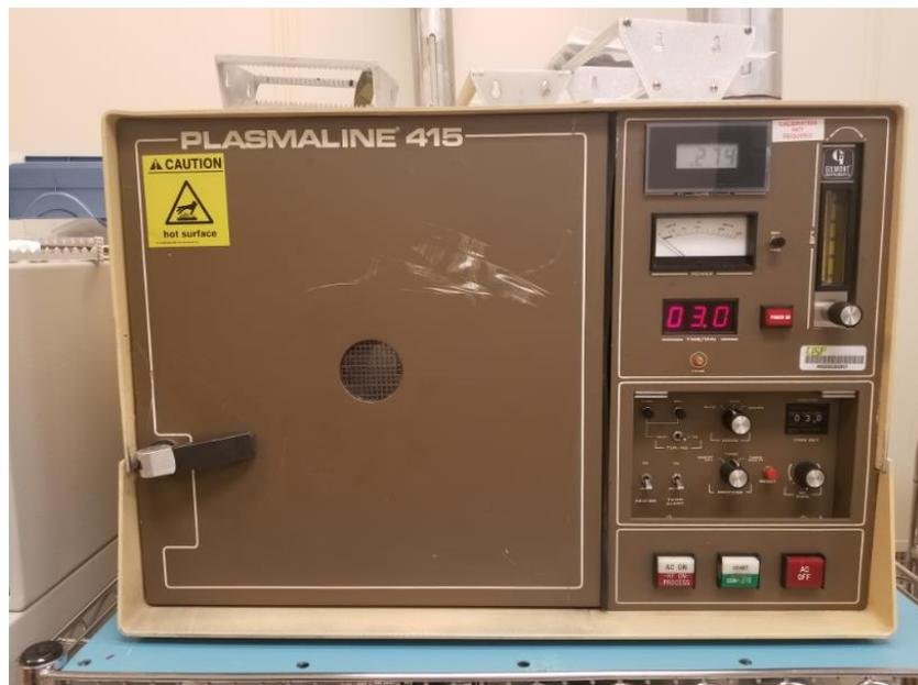
Figure 16: Plasmaline 415 for removing organic compounds after DRIE etch
