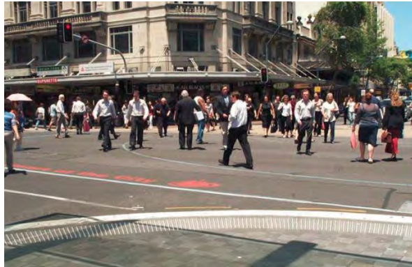
Figure 5 Exclusive pedestrian signal phase - scramble phase (extracted from NZ transport agency 2009)
