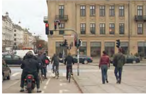
At intersection, bicycle light and 1.5 meter lane is provided for both straight and right- turning cyclists
