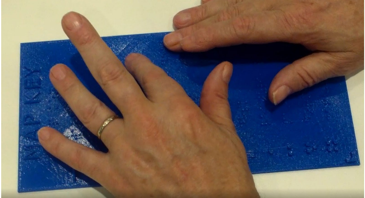
Figure 3.6 3D-printed tactile map key with a sharp braille and rough background surface.
