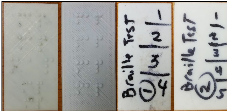
Figure 3.2 3D-printed Braille test plates with different dot styles and parameters.
