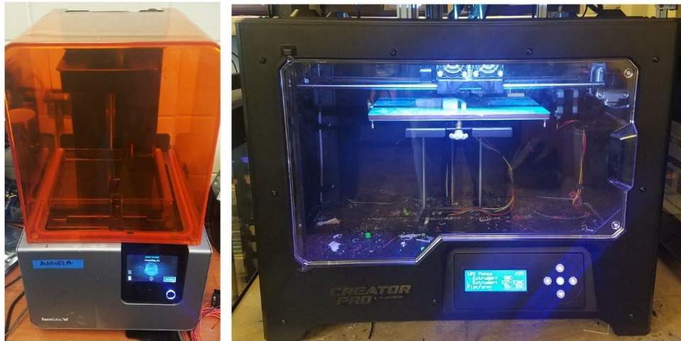
Figure 2.4 Left) a Formlabs Form 2 SLA 3D-printer. Right) a FlashForge Creator Pro FDM 3D-printer. Photographs taken by Howard Kaplan, at the University of South Florida, Advanced Visualization Center 3D-Printing Lab 01.31.2019.
