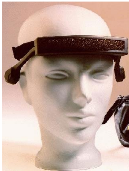
Figure 2.3 Sonic Pathfinder, a head-mounted pulse-echo sonar system controlled by a microcomputer for out-of-door object detection. Used with permission from Tony Heyes Ph.D.
