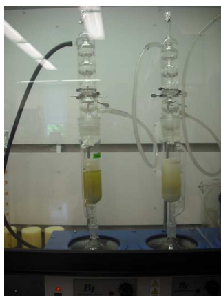
Figure 9. The set up of two Soxhlet extractors on heating mantles with power on, in the laboratory, is shown for C. virginica samples collected at Ruskin and the Upper Tampa Bay Park, Florida (a). The rotary evaporator set up, with connection to a cold water source to feed into the coils, in addition to connect to the motor for production of the vacuum (b).
