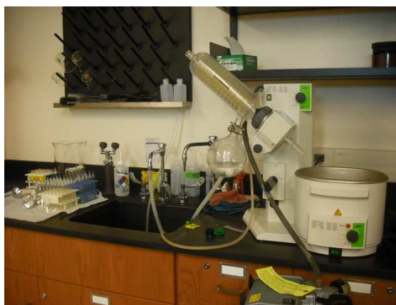
Figure 9. The set up of two Soxhlet extractors on heating mantles with power on, in the laboratory, is shown for C. virginica samples collected at Ruskin and the Upper Tampa Bay Park, Florida (a). The rotary evaporator set up, with connection to a cold water source to feed into the coils, in addition to connect to the motor for production of the vacuum (b).
