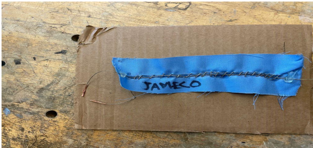
Figure 5.1 JAMECO Fiber-based Supercapacitor (Hand Stitching Technique).
