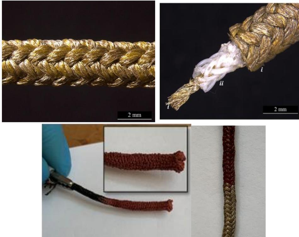
Figure 27. a) Triaxial braided piezo fiber, b) braided PVDF with inner silver coated nylon, c) triaxial braided piezo fiber with MWCNTs ink used for the hydrogen evolution assisted electroplating showing a higher porosity structure, d) triaxial braided piezo fiber without MWCNTs after deposition
