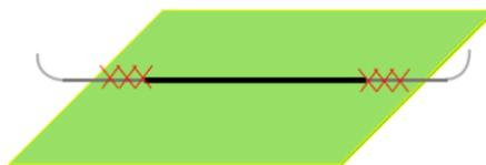
Figure 13. A schematic of a piece of fabric with MWCNT track and connection cables properly sewed to provide continuous connection between the fabric and the instrument.
