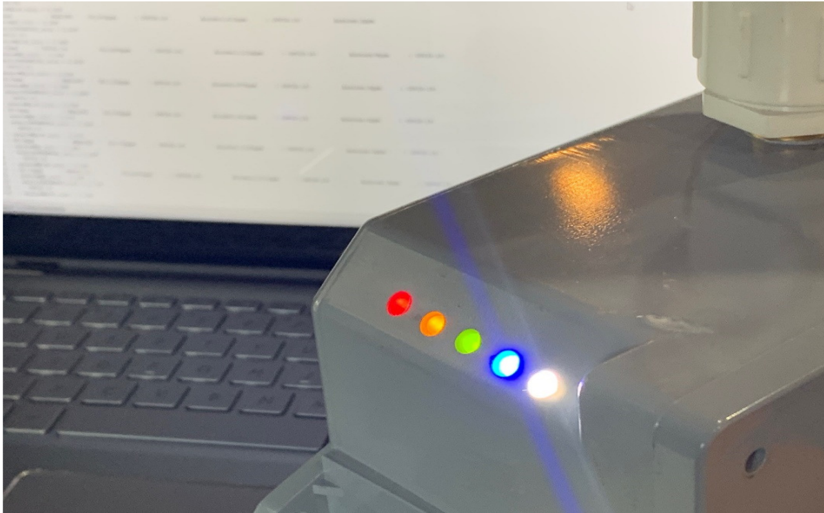
Figure 3.4 The electronic nose testbed prototype housing has LEDs illuminating in response to predetermined threshold levels of target gas concentration in ppm.
